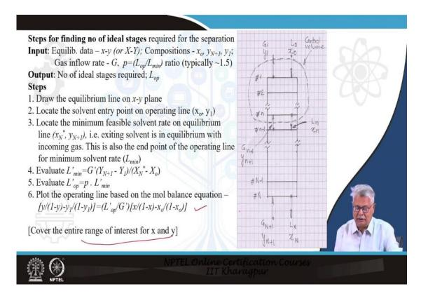
Here the same thing is written stepwise in a set of instructions. What we have is basically how to plot the operating line and it has to cover the entire range of interest for x and y for x naturally its  $x_0$  to your  $x_N^*$ .
