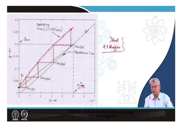
Here what we have is a x y coordinate here we have is the y and here we have the x, the equilibrium data is here. The corresponding to the  $L'_{min}$  is my starting point which is the top of my absorber and this is the bottom end and we have noted that corresponding to  $y_{N+1}$ . What we have here is basically  $x_N^*$ .
