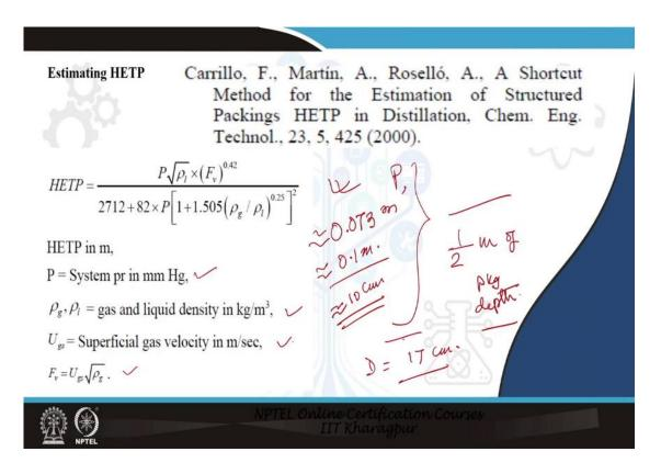
HETP is found from various correlations, but for vapour-liquid contacting there is a simplified method which is published in 2000 and it goes like this, it involves a pressure of the column it is for a low-pressure column. P is a system pressure in millimetre mercury,  $\rho_g$  and  $\rho_l$  are gas and liquid density in kg per meter cube,  $U_{gs}$  is a superficial gas velocity in m/s and  $F_v$  is  $U_{gs}\sqrt{\rho_g}$ .
