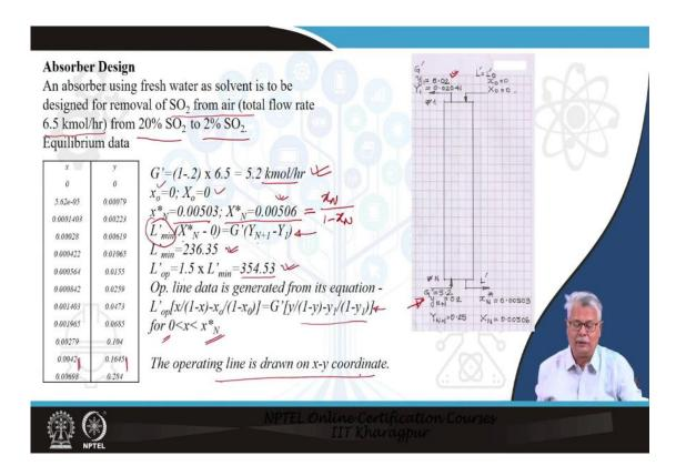
We have a case of an absorber design example with us. The absorber is using freshwater as a solvent for the removal of  $SO_2$  from the air, the total flow rate of the air is 6.5 kmol/h and it has got 20%  $SO_2$ . So, quite naturally 20% of  $SO_2$  is 1.3 kmol/h  $SO_2$  and the rest amount is inert air and it is brought down to 2 %  $SO_2$ .
