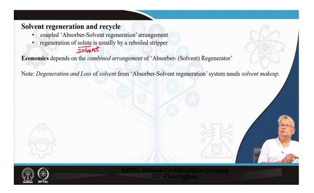
You have the solvent regeneration and recycle arrangement. It is an integral part of the absorption system. Absorption, where the absorber-solvent regeneration arrangement acts as a coupled system. The regeneration of the solute is usually done by a revolt stripper. It is the regeneration of the solute as well as the regeneration of the solvent itself, both are true.
