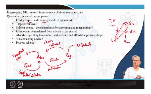
Here, we have an example and perhaps more details regarding the design, we try to frame while discussing this example itself. It is almost the same example here, which is ammonia removal from a stream of air ammonia mixture; that means, my air-stream is contaminated with ammonia. Possibly it has been picked up during a process and when I went out my air to the open atmosphere, I need to remove this ammonia.
