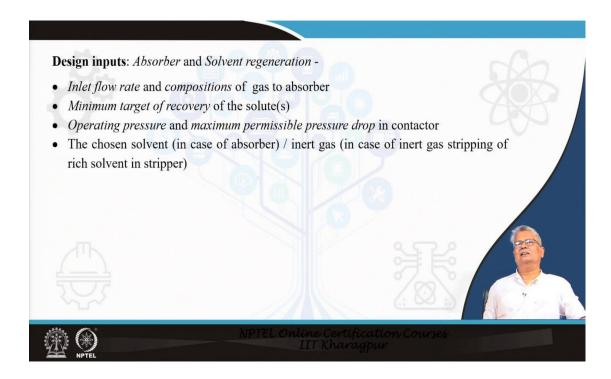
If you look at the design inputs, the flow rates, the minimum target of recovery, the pressure and the chosen solvent are the design inputs.
