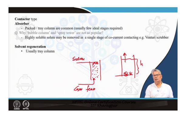
Now, we focus on the contactor type. We usually have packed or tray columns. These primarily require a few ideal stages only. We will look at the details of these trays and the columns packed slightly later on possibly in the next class. I have a question here why not have a column which is filled with liquid, have a sparger at the bottom and let the bubble go out; that means, it is a bubble columned, why bubble columns are not popular?
