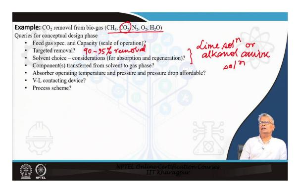
We have here another example with us. It is the CO<sub>2</sub> removal from the biogas. In fact, if you have biogas production, normally the gas that you will be producing will be a mixture of a good amount of methane fair amount of CO<sub>2</sub>, a small amount of nitrogen-oxygen and it will be moist. If we try to handle this and we think of removing the CO<sub>2</sub> part of it primarily, we have to face the same questions and we go for the conceptual design by following the steps.
