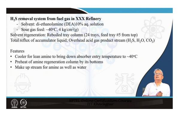
We have here another example in which we have a removal system from  $H_2S$  removal system from a fuel gas in a typical refinery. This example is from real life. This refinery uses 10% aqueous solution of diethanolamine. The sour gas feed is at a temperature of around 40 °C and a pressure of around 4 kg/cm<sup>2</sup> gauge. The absorber in this particular case is a packed tower.
