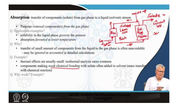
Let us look at the process of absorption itself. Absorption means a process in which we have some components which are present at a gas phase and they will get transferred to a liquid phase which is brought in contact with a gas phase. The liquid phase is called typically solvent and the transferred component is called the solute because it is more
