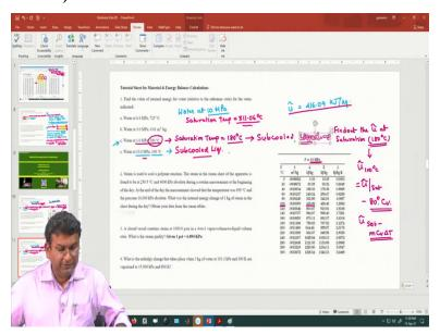
We should go to the steam table and from the steam table if we go to the pressure side table, we see that at 10 MPa the temperature the saturation temperature is 311°C. So, this is what you can see. And so, water at 10 MPa the saturation temperature is 311°C therefore what we have is a sub
