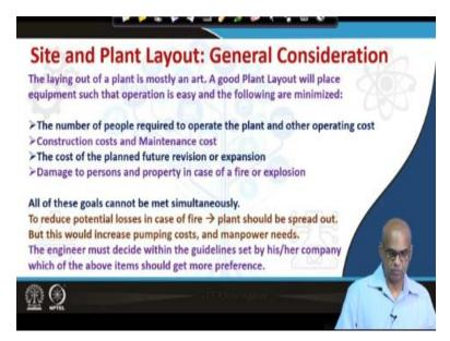
The laying out of a plan is mostly an art, a good plant layout will place equipment such that operation is easy and the following are minimized. The number of people required to operate the plan and the other operating cost. Construction cost and maintenance cost, the cost of the planned future revision or expansion, damage to persons and property in case of a fire or explosion. All of these goals cannot be made simultaneously.
