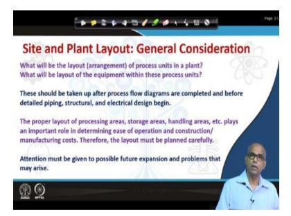
So, as I told you now you have determined the location of the plant, you have the flow sheet with you, so now you are going to decide what will be the layout or arrangement of process units in the plant, what will be the layout of the equipment within these processing units? So this should be taken up after process flow diagrams are completed and before detail piping, structural, and electrical design begin.
