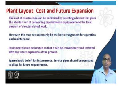
These are the factors that do not need to be considered for plant layout based on cost and scope for future expansion. The cost of construction can be minimized by selecting a layout that gives the shortest run of connecting pipe between equipment and the list amount of structural steel work. However, these may not necessarily be the best arrangement for operation and maintenance.
