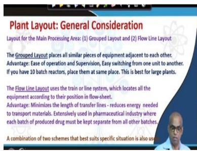
Now, we will talk about Plant Layout. There are two types of plant layouts group layout and flow line layout. The group layout places all similar pieces of equipment at one place. So, all similar pieces of equipment will be placed adjacent to each other. So, what is the advantage? This leads to ease of operation, ease of supervision also it is easy to switch from one unit to
