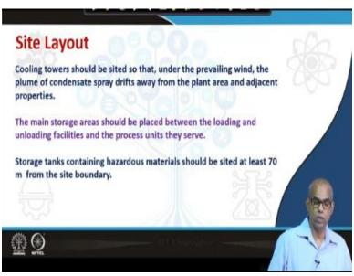
Cooling towers should be cited so that, under the prevailing wind, the plume of condensate spray drifts away from the plant area and adjacent properties. The main storage areas should be placed between the loading and unloading facilities and the process units they serve. Storage tanks containing hazardous materials should be cited, at least 70 meter from the site boundary.
