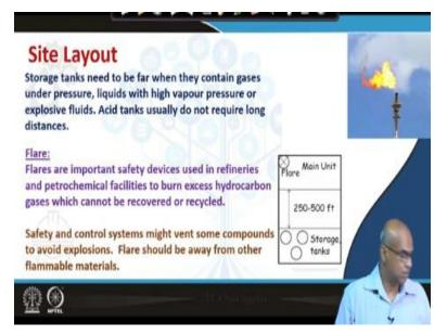
Storage tanks needed to be far when they content gases under pressure, liquids with high vapour pressure or explosive fluids. Acid tanks usually do not take long distance. What you see here, is another simple schematic of the site layout. So, these are the storage tanks on one end. Now between the storage tank and the main unit there is about 250 to 500 feet distance meaning about 70 meter to about say 170 meter distance.
