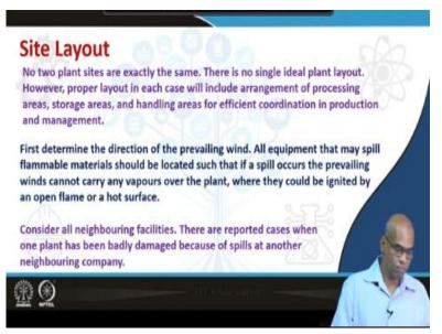
No two plants are exactly the same. Because most probably no two plants will be exactly same and no two plants sites will also never be exactly the same. So, there is no single ideal plant layout. However, proper layout in each case will include arrangement of processing areas, storage areas and handling areas for efficient coordination in production as well as management. First determine the direction of the prevailing wind.
