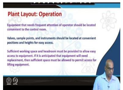
These are the factors based on ease of operation. Equipment that need frequent attention of operators should be located convenient to the control room. Valves, sample points and instruments should be located at convenient positions and heights for easy access. Sufficient working space and headroom must be provided to allow easy access to equipment. If it is anticipated that equipment will need replacement then sufficient space must be allowed to permit access to lifting equipment.
