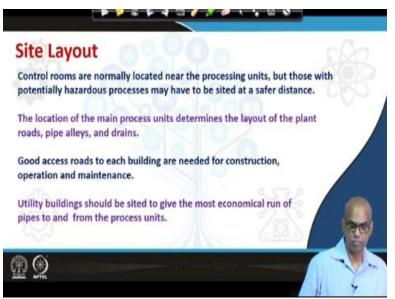
Control rooms are normally located near the processing units, but those with potentially hazardous processes may have to be cited at a safer distance. The location of the main process units determines the layout of the plant roads, pipe alleys and drains. Good access roads to each building are needed for construction operation and maintenance. Utility buildings should be cited to give the most economical run of pipes to and from the process units.
