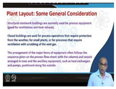
Before that let us talk about some general consideration. Structural steel work buildings are normally used for process equipment because they are good for ventilation and heat release. Close buildings are used for process operations that require protection from the weather for small plants or for processes that require ventilation with scrubbing of the vain gas. The arrangement of the measure items of equipment often follows the sequence given on the process flow sheet;
