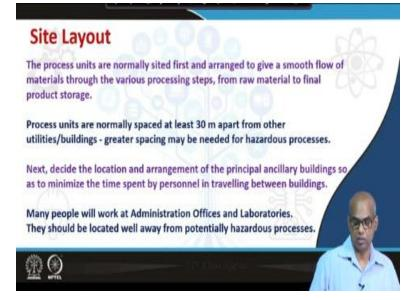
The process units are normally cited past and arrange to give a smooth flow of materials through the various processing steps from raw material to final finish product storage. Process units are normally spaced at least 30 meter effort from other utilities or buildings, greater spacing must be needed for hazardous processes. Next decide the location and arrangement of the principle ancillary buildings, so as to minimize the time span by personnel in travelling between the buildings.
