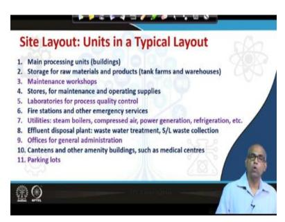
So, these are the typical units that you will be placing in a layout. Main processing units, storage for raw materials and products; this will be tank farms and warehouses, maintenance workshop, stores, for maintenance and operating supplies, Laboratories for process quality control, Fire stations and other emergencies services, Utilities: such as steam boilers, compressed air, power generation, refrigeration, etcetera.
