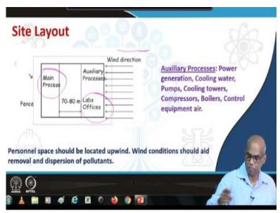
What you see is a very simple schematic of a site layout. Look at the wind direction so, the occupied buildings such as labs offices, these are occupied by human. So, occupied buildings are located such that, the wind conditions will aid removal and dispersion of pollutants. So this is the main process and there is about 70 to 80 meters distance between these occupied buildings and the main process.
