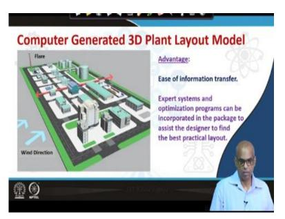
So this is a computer generated 3 D plant layout model. So look at the wind direction, you have the offices near the main entrance, you have the storage tanks, you have the flare. So the layout conforms to whatever we discussed as factors that we consider. So if you generate models for plant layout using computers software's, it becomes very easy to transfer this information say to your colleague.
