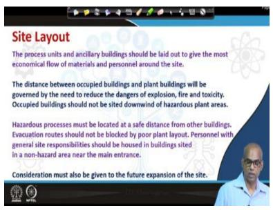
The process units and ancillary buildings should be laid out to give the most economical flow of materials and personnel around the site. The distance between occupied buildings and plant buildings will be governed by the need to reduce the dangers of explosion fire and toxicity. Occupied buildings should not be cited downwind of hazardous plant areas. I repeat occupied buildings should not be cited downwind of hazardous plant areas, there should be cited upwind.
