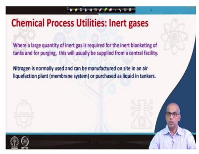
Next, we move on to inert gases where a large quantity of inert gas is required for the inert blanketing of tanks and for purging, this will usually be supplied from central facility. So inert gas is used to have an inert environment. It will be required for the inert blanketing of tanks and for purging. Nitrogen is normally used and can be manufactured on site in an air liquefaction plant or it may also be purchased as liquid nitrogen in tankers from utility supply companies.
