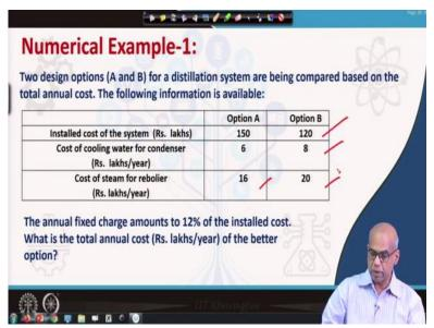
Now, let us take a simple example. We have two design options: option A and option B for a distillation system and these two options are being compared based on the total annual cost. We have the following information's available as shown in the table. Installed cost of the system is 15000000 for option A and 12000000 for option B. Cost of cooling water for condenser in lakhs per year for option A is 6 and for option B is 8.
