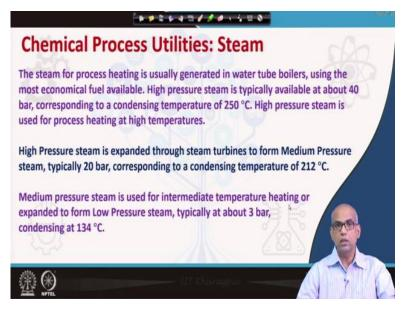
The steam for process heating is usually generated in water tube boilers using the most economical fuel that is available. High pressure steam is typically available at above 40 bar corresponding to a condensing temperature up to 250 degree Celsius. High pressure steam is used for process heating at high temperatures. High pressure steam is expanded through steam turbines to form medium pressure steam, typically at 20 bar, corresponding to a condensing temperature of 212 degree Celsius.
