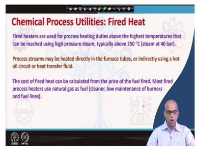
Now let us move on to next utilities - fired heat. Fired heaters are used for process heating duties above the highest temperature that can be reached using high pressure steam typically above 250 degree Celsius using steam at 40 bar. Process streams may be heated directly in the furnace tubes or indirectly using a hot oil circuit or heat transfer fluid. The cost of fired heat can be calculated from the price of the fuel fired.
