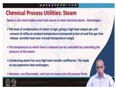
Steam is the most widely used heat sources in most chemical plants. So steam is the very very important process utility. It has several advantages such as the heat of condensation of steam is high giving a high heat output per unit amount of utility at constant temperature compared to hot oil and flue gas that release sensible heat over a broad range of temperature. The temperature at which heat is released can be controlled by controlling the pressure of the steam.
