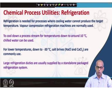
Now let us move on to refrigeration. Refrigeration is needed for processes where cooling water cannot produce the target temperature. Vapour compression refrigeration machines are normally used. To cool down a process stream for temperatures down to around 10 degree Celsius, chilled water can be used. For further lower temperatures, say down to -30 degrees Celsius, salt brines, sodium chloride, calcium chloride are commonly used.
