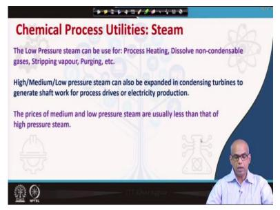
The low pressure steam can be used for process heating, dissolve non-condensable gases, stripping vapour, purging etcetera. High pressure steam, medium pressure steam or low pressure steam can also be expanded in condensing turbines to generate shaft work for process drives or electricity production. The prices of medium and low pressure steam are usually less than the price of high pressure steam.
