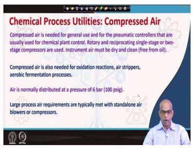
Now, let us move on to compressed air. Compressed air is needed for general use and for the pneumatic controllers that are usually used for chemical plant control. In chemical process industries pneumatic controllers are routinely used. So, pneumatic controllers will receive pneumatic signal. So you will need compressed air for that purpose. Rotary and reciprocating
