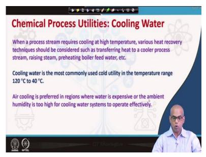
Let us now move on to next utility cooling water. When a process stream requires cooling at high temperature, you must consider various heat recovery techniques such as transferring heat to a cooler process stream, raising steam, preheating boiler feed water etc. So the heat must be reused. Cooling water is the most commonly used cold utility in the temperature range of 120 degree Celsius to 40 degree Celsius.
