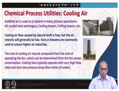
Now let us move on to cooling air. Ambient air is caused;, ambient air is used as a coolant in many process operations. For example, air cooled heat exchanger, cooling towers, prilling towers is used in urea manufacture. So ambient air is used as a coolant in several important process operations such as heat exchangers, cooling towers, prilling towers etcetera. Cooling air flow caused by natural draft is free, but the air velocity will generally be quite low.
