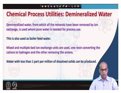
Demineralized water, from which all the minerals have been removed by ion exchange, is used where pure water is needed for process. This is also used for boiler feed water. Mixed and multiple-bed ion-exchange units are used one resin converting the cations to hydrogen and the other removing the anions. Water with less than 1 part per million of dissolving solids can be produced.
