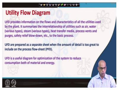
Now, we have talked about various chemical engineering flow diagrams such as block flow diagrams, process flow diagrams, piping an instrumentation diagram. Chemical engineers also use utility flow diagram. Utility flow diagram provides information on the flows and characteristic of all the utilities used by the plant. It summarizes the interrelationship of utilities
