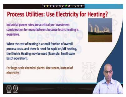
Should we use electricity for heating in industry? Industrial power rates are a critical preinvestment consideration for manufacturers because electric heating is expensive. When the cost of heating is small fraction of overall process costs and there is need for rapid on/off heating, the electric heating may be used. For example, small scale batch operations for large scale chemical plants, better we should use steam instead of electricity for heating.
