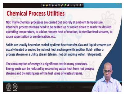
Not many chemical processes are carried out entirely at ambient temperature. They are carried out at various temperatures depending on what temperature will be the optimum temperature for the particular process. So routinely process streams need to be heated up or pulled down to reach the desired operating temperature to add or remove heat of reaction, to sterilize feed streams or to cause vaporization or condensation etcetera.
