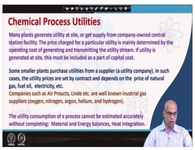
Many plants generate utility at site or get supply from company-owned central station facility. The price charged for a particular utility is mainly determined by the operating cost of generating and transmitting the utility stream. The utility is generated at site, this must be included as part of capital cost. So any utility is generated at site, you must include this as part of capital cost. Some smaller plants purchase utilities from a utility company.
