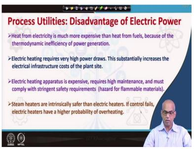
There are certain disadvantages of using electric power heat from electricity is much more expensive than heat from fuels because of the thermodynamic inefficiency of power generation. Electric heating requires very high power draws. This substantially increases the electrical infrastructure cost of the plant site. Electric heating apparatus are expensive, requires high maintenance and must comply with very stringent safety requirements.
