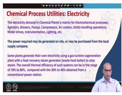
Now, let us talk about individual utilities in some more details. Let us start with electricity. The electricity demand in chemical plants is mainly for electrochemical processes, Agitators, Blowers, Pumps, Compressors, Air coolers, Solids-handling operations, Motor drives, Instrumentation, Lighting etc. The power required may be generated on site or may be purchased from the local supply company.
