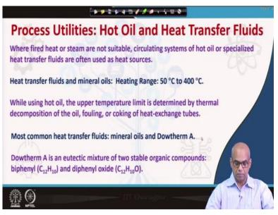
Now let us move on to hot oil and heat transfer fluids. Where fired heat or steam are not suitable, circulating systems of hot oil or specialized heat transfer fluids are often used as heat sources. So there will be circulating system of hot oil or specialized heat transfer fluids. Heat transfer fluids and mineral oils are typically used for heating in the range of 50 degree Celsius to 400 degree Celsius.
