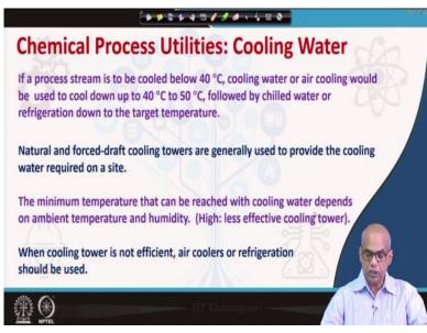
If a process stream is to be cooled below 40 degree Celsius, cooling water or air cooling would
