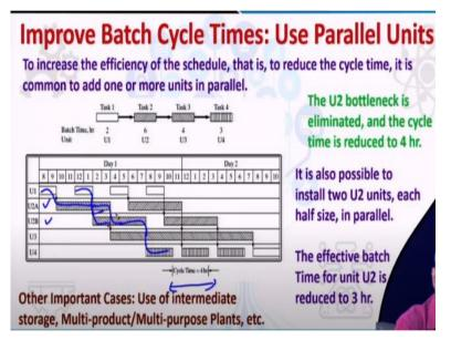
But here we improve the schedule by making use of fewer pieces of equipment. We could release U4. We can also improve the batch cycle times or the schedule by using parallel units. So in this particular case, where we use two parallel units of U2, U2A and U2B. And you notice that the cycle time has reduced from 6 hours to 4 hours. Note that this is my first batch and this is the second batch. (**FL**).
