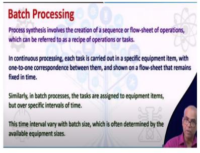
Process synthesis involves the creation of a sequence or flow sheet of operations, which can be referred to as the recipe of operations or task. In continuous processing, we know that each task is carried out in a specific equipment with one to one correspondence between them. And this piece of equipment is shown on a flow sheet that remains permanently fixed as long as the operation is on.
