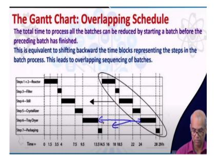
So we will talk about so we think of overlapping schedule. In overlapping schedule the total time of the processes, the total time to process all the batches can be reduced by starting a batch before the preceding batch has finished. That means, we do not have to wait up to this point all the time to start the next batch. We can start a batch before the preceding batch has finished.
