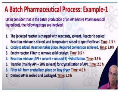
Let us take an example first. As a batch process, let us consider a pharmaceutical process, which is manufacturing an active pharmaceutical ingredient, which you call API. So active pharmaceutical ingredient is the key component is the main component
