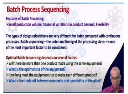
As we have talked about before, that there are several distinct features of batch processing or batch processes which makes it different from continuous processing. For example, for large volume processing we will always go for continuous processes, but for small production volume for example, small volume high value pharmaceutical products or specialty chemicals we will go for batch processing.
