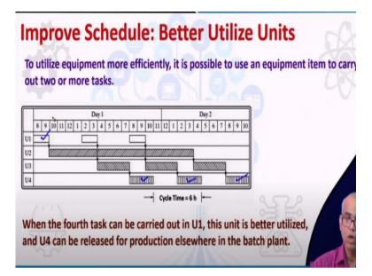
Now can I improve this schedule further? To utilize equipment more efficiently it is possible to use an equipment item to carry out two or more task. As of now we have been using each equipment for a dedicated task. Now if an equipment is available, if it is idle, and if it is possible to carry to carry out the task of another equipment in this particular equipment that is free, we should better do that and can release or can free up the other equipment.
