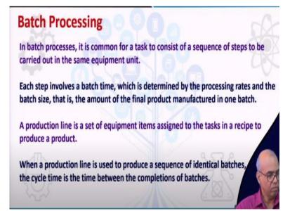
In batch processes, it is common for a task to consist of a sequence of steps to be carried out in the same equipment unit. Each step involves a batch time, which is determined by the processing rates and the batch size, which is the amount of the final product manufactured in one batch. A production line is a set of equipment items assigned to the task in a recipe to produce a product.
