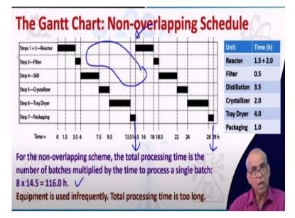
So let us first look at non-overlapping schedule. Note that this chart shows that I am done here with the first batch, 14.5 hours. So the Gantt chart shows that 14.5 hours my first batch is over and the second batch also starts at 14.5, which is again over after another 14.5 hours that means 29 hour. So it takes 29 hour to produce or complete two batches. So the non-overlapping schedule is represented on the Gantt chart by simply repeating the sequence one after another.
