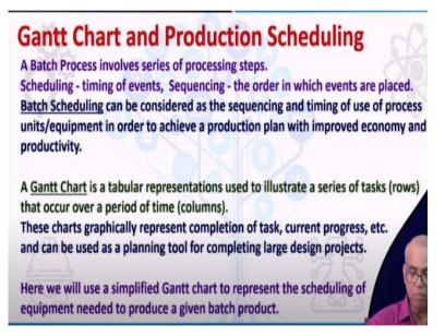
A batch process involves series of processing steps. It is like a recipe based operation. So there are series of events that will take place, a series of processing steps, welldefined series of processing steps. Scheduling means timing of these events and sequencing means, the order in which the events are placed or the order in which these events will occur. So scheduling means timing of events and sequencing means the order in which these events will occur.
