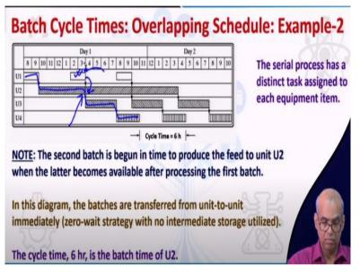
You notice that well, this represents the first batch. The second batch has begun in time to produce the feed to unit 2 when unit 2 is available after processing the first batch. So unit 2 is completed here. So U1 has started in time, so that it can give feed to U2 in time. Of course here again, we are assuming zero-wait strategy and also there is no intermediate storage. The cycle time is 6 hours.
