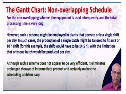
Now this non-overlapping schedule, which of course is not very efficient in the sense that the equipment is used infrequently and the total processing time is unnecessarily long. But it has certain advantages as well. Such a scheme might be employed in plants that operate only a single shift per day. In such case, what we will do is the production of a single batch can be tailored to fit an 8 hours or 10 hour shift.
