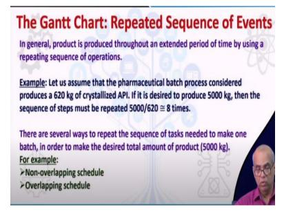
Now in general, a product is produced throughout an extended period of time by using a repeated sequence of operations. You are not going to use only one sequence of this process. Depending on how much of API you want to produce, you have to repeat this sequence of batch processes. For example, let us assume that the batch process that we are considering produces 620 kg of crystallized API in one batch and let us say my target is to produce 5000 kg of this API.
