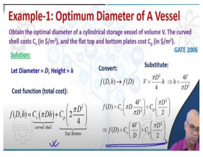
So let us take the first example, which is the determination of optimum diameter for a vessel. Obtain the optimal diameter of a cylindrical storage vessel of volume V. The current shell cost C s in dollar per meter square and the flat top and bottom plates cost C p in dollar per meter square. So you have to find out the optimal diameter of the cylindrical storage vessel of specified volume V.
