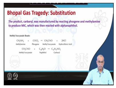
Substitution; the product carbaryl which is an insecticide was manufactured by reacting phosgene and methylamine. So, methylamine and phosgene were reacted to produce methyl isocyanate and hydrochloric acid. Methyl isocyanate is the intermediate which is a deadly gas. So methyl isocyanate was reacted in the next step with alpha naphthol to produce the product carbaryl which is used as insecticide.
