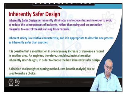
Inherently safer design permanently eliminates and reduces hazards in order to avoid or reduce the consequences of incidence rather than using add-on protection measures to control the risk arising from hazards. Inherent safety is the relative characteristic and it is appropriate to describe one process as inherently safer than another. It is possible that a modification in 1 area may increase the hazard in another area or it may also decrease hazard in another area.
