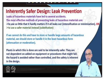
Now, let us try to understand the basics of inherently separate design by taking an example of leak prevention. Note that leaks of hazardous materials have led to several accidents. The most effective method of preventing leaks of hazardous materials are to use so little of the hazardous material that it will not matter at all if everything leaks out. Everything in the sense the if all the hazardous materials leaks out then also perhaps it will not cause a disaster.
