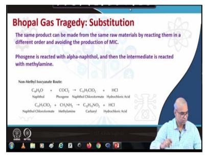
So non-methyl isocyanate route. The same product carbaryl can be made from the same raw materials, phosgene and methylamine. By reacting them in a different order. And thereby avoiding the production of methyl isocyanate, how? So this is the non-methyl, non-methyl isocyanate route. So in this case phosgene is first reacted with alpha-naphthol. Look at the reaction is now being carried out in a different order.
