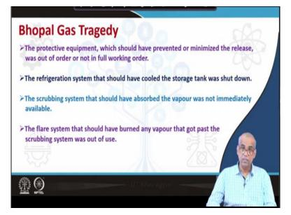
The protective equipment which should have prevented or minimized the release or methyl isocyanate was out of order or not in full working order. The refrigeration system that should have cooled the storage tank was shut down. A serious lapse of safety measure. The scrubbing system that should have absorbed the vapour was not immediately available. Another lapse of safety measure.
