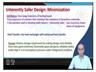
Distillation column uses large inventory or boiling liquids. So when you are using a sequence of distillation columns to perform the separation of multi component mixtures, let us use sequence of columns that minimize the inventory of hazardous materials. So these objectives can be included in the design of distillation sequence. We can use partition wall or dividing wall column.
