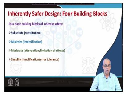
Now among these various inherent safety principles 4 building blocks are very, very important. Those four basic building blocks of inherent safety are substitution, intensification, attenuation or moderation and simplification. And we can also consider that this is the hierarchy in which we should approach inherently safer design. For example, we should look at the principle of substitution first, then intensification, then moderation and then simplification.
