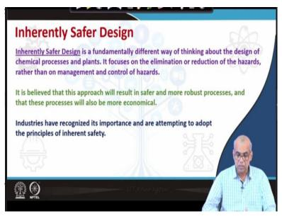
Inherently safer design is the fundamentally different way of thinking about the design of chemical process. As we just discussed, the inherently separate design focuses on the complete elimination or significant reduction of hazards instead of managing and controlling the hazards. We can apparently think such design processes will lead to very expensive plants. But on the contrary it is generally believed that this approach will result in economical processes, it will be safer and more robust.
