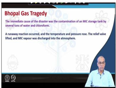
The immediate cause of the disaster was the contamination of an methyl isocyanate storage tank by several tons of water and chloroform. A runaway reaction occurred and the temperature and pressure rose. They rose to very high extent. The relief valve lifted and the methyl isocyanate vapour was discharged into the atmosphere. Unfortunately, the protective equipments were either absent or was not in full working order.
