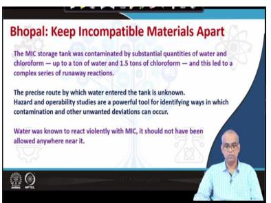
We should keep incompatible material apart. The methyl isocyanate storage tank was contaminated by substantial quantities of water and chloroform. It is estimated that a ton of water and one and half ton of chloroform was mixed with methyl isocyanate storage tank. And this led to a complex series of runaway reaction. The precise route by which water entered the tank is unknown.
