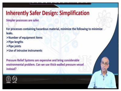
Finally, the last principle is simplification. Simpler processes are always safer. For processes
