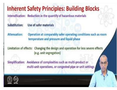
Now, apart from intensification, substitution, attenuation we have several principles that are used in inherently safer design. So, you can call them inherent safety principles or building blocks of the inherently safer design. For example, intensification means reduction in the quantity of hazardous materials, substitution means use of separate materials. We show these when we talk about leak prevention example.
