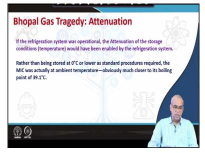
Next attenuation or moderation: If the refrigeration system was operational, the attenuation or moderation of the storage conditions that means the temperature of the storage tank would have been enabled by the refrigeration system. Note that it is a standard procedure to store such liquid at 0 degree Celsius or even at lower temperature. But the methyl isocyanate was actually stored at ambient temperature. And the ambient temperature was much closer to its boiling point of 39.1 degree Celsius.
