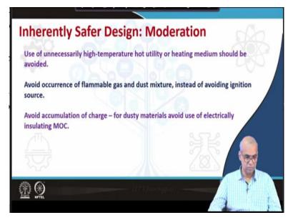
Next principle in the hierarchies moderation or attenuation. Use of unnecessarily high temperature hot utility or heating medium should be avoided. Avoid occurrence of flammable gas and dust mixture instead of avoiding ignition sources. There are large numbers of ignition sources, so you should more rely on avoiding occurrence of flammable gas and dust mixtures. Avoid accumulation of charge.
