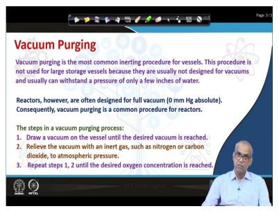
Vaccum purging is the most common inerting procedure for vessels this procedure is not used for large storage vessels because they are usually not designed for vacuums and usually can withstand a pressure of only few inches of water. However, reactors are often designed for full vacuum that means zero millimeter a mercury absolute. Therefore the vacuum purging is common procedure for reactors. The steps in a vacuum purging process are as follows.
