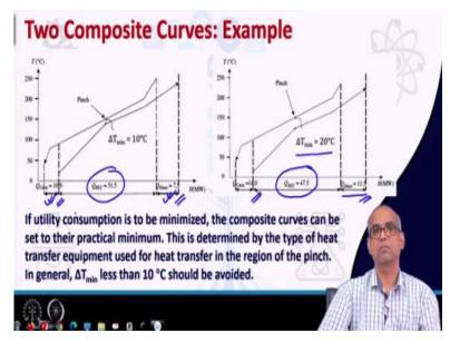
Now, let us take back that example and find out these composite curves for two different delta T minimum; one is 10 degrees celsius and this source for 20 degree Celsius. Look at the pinch points, for the first case where the delta T minimum is set to 10 degrees Celsius. So delta T the 10 degree Celsius is obtained here. So this is 10 degree Celsius, the pinch point. In this case the amount of heat recovery is 51.5 megawatt.
