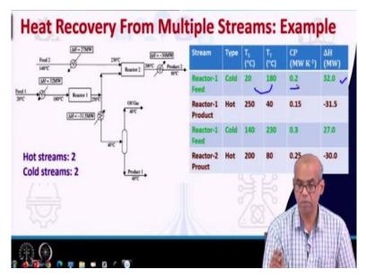
Now, let us take an example to understand these concepts where we will have the temperature and the enthalpy values taken from a simple process flow sheet. So consider this simple flow sheet for a process where you have two reactors and one separator. In this example the temperature and enthalpy values for the streams are shown. There are two hot streams, what are those hot streams?
