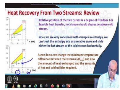
Let us first quickly review what you have learnt for two stream systems. Now look at the temperature enthalpy diagram on which one hot stream and one cold stream we have plotted. The hot streams have been plotted from its supply temperature to target temperature and also the cold streams have been plotted from its supply temperature to its target temperature. We also know that slope of this curve is 1 by CP where CP is the heat capacity flow rate.
