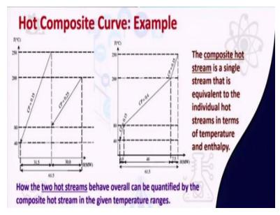
So we have now first plotted the hot streams. So what was the temperature of the two hot streams? One is 250 to 40 another was 200 to 80. So, we plot first hot stream 250 to 40 and 200 to 800, their CP values are also shown. So you can have more number of streams here. But the way we form the hot composite curve will be exactly same. Now how the two hot streams behave overall can be quantified by the composite hot stream in the given temperature range.
