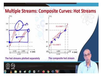
Now, let us consider how we construct a hot composite curve from these two individual hot streams. So the first hot stream has CP value of 15 kilowatt per degree Celsius and the other one has CP value of 25 kilowatt per degree Celsius. Note that in this temperature interval only 1 hot stream is working. So depending on the starting and ending of the streams. We have divided this temperature scale into temperature intervals.
