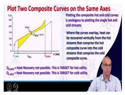
Now let us plot this two composite curves on the same axis, like in case of two stream problems, we plot it, the hot stream and the cold stream I had only one hot stream, I had only one cold stream so I plot in the hot stream and cold stream on the temperature enthalpy diagram and can infer the heat recovery and the heat duties for the, utilities or the loads for the utilities. So, I follow the same approach.
