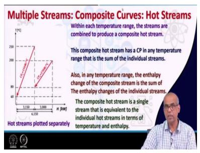
So let us look at this example, where we have plotted two hot streams on this temperature enthalpy diagram. So, two hot streams are plotted separately on this temperature and therapy diagram. Note, that depending on the starting or ending of the streams we have divided this temperature scale into various ranges. So we have now several temperature ranges. Here we have one temperature range and there is only one stream working only this stream.
