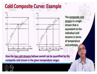
Exactly same way let us now find out the cold composite curve and the cold composite curve will be equivalent to the individual cold composite, cold streams in terms of temperature and enthalpy.
