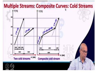
Exactly the same way we can find out the composite curve for cold streams. Again, we add up the CP values in each temperature range. So in this temperature range I have only one CP value which is 20, again in this temperature range I have one CP value, which is 20. But in these temperature ranges I have 2 CP values for 2 streams, which is 20 + 60 is 80. So, exactly the same way you can obtain the composite curve for cold streams and we will call that, cold composite curve.
