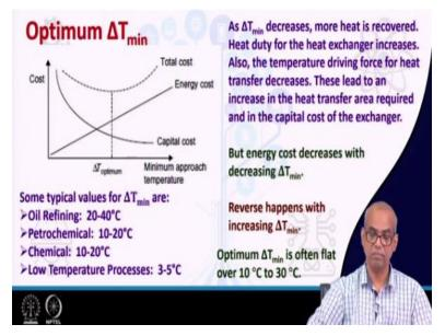
When you decrease the delta T minimum values we see that there is greater degree of overlap between the two composite curves. So, thus more and more amount of heat will be recovered. So when more amount of heat needs to be recovered will be recovered heat duty for the heat exchanger will increase. But you also see that the driving force for heat transfer decreases delta T minimum decreases, driving force for heat transfer decreases.
