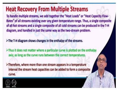
Now let us see how do I explain these concepts to heat recovery from multiple streams? To handle multiple streams, we simply add together the heat capacity flow rates of all streams existing over any given temperature range. So what we do is, we will plot all the individual streams. Let us say first let us talk about hot streams. So, all the individual hot streams will be plotted on the temperature versus enthalpy diagram.
