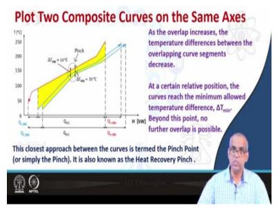
The larger the; value of the delta T minimum the smaller the possible maximum heat recovery. Note that the delta T minimum as you see in this figure will be larger by sliding the cold stream to the right hand side. So this will decrease the region of overlapping between these two composite streams. So, that is why the larger the value of the delta T minimum the smaller the possible maximum heat recovery.
