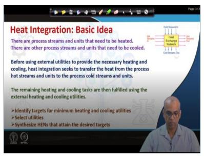
Now, what is the basic idea of heat integration? In any chemical process industry, there are process streams and units that needs to be heated. And also, there are other process streams and units which needs to be cooled down. Of course, you can make use of stream utility to heat up those process streams which needs to be heated. And for the cooling you may need cooling utility. But that will invite more cost.
