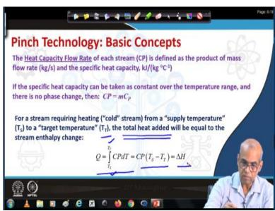
We will define one more term known as heat capacity flow rate. Heat capacity flow rate of each stream is defined as the mass flow rate of that stream multiplied by the specific heat capacity of that stream. See the specific heat capacity is taken as constant say over the temperature range of supply to the final temperature. So, initial temperature between initial temperature and the final temperature if the specific heat capacity is considered constant.
