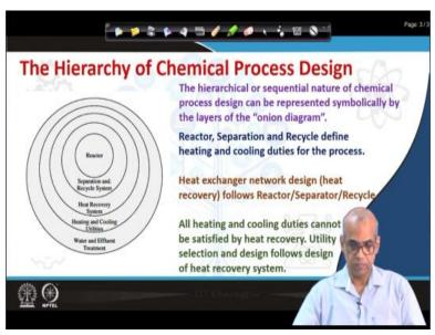
This is the only end diagram which shows the hierarchical nature of the chemical process design. Chemical reactor is often the heart of any chemical process and the design activity starts with the design of the chemical reactor. Next comes the design of separation and recycle. Once you have designed the reactor separation system and recycle, you have finalized your mass and energy balance.
