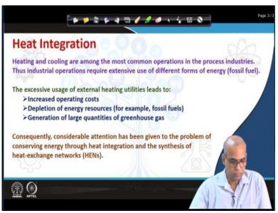
As we just discussed heating and cooling are among the most common operations in the chemical process industries. Industrial operations require extensive use of different forms of energy, such as safe fossil fuel. The excessive uses of external heating utilities will lead to
