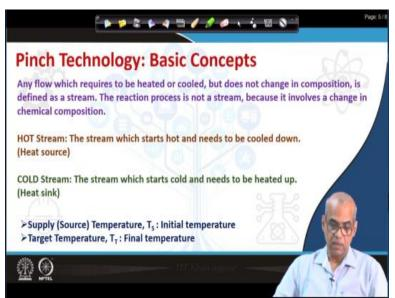
Now, let us define certain terms any flow which requires to be heated or cooled but does not change in composition is define as a stream. So, stream is any flow which requires to be heated up or cool down. But it does not change in composition. So, in the previous example, the chemical reactor is not a stream because there is a change in composition within the reactor. But the feed stream and the products in their streams that is why we are talking about feed stream coke and the product stream.
