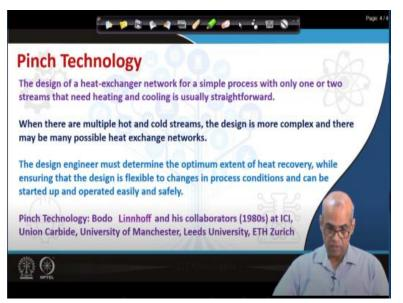
Now we will start the introduction to pinch technology as a method for heat integration. The design of a heat exchanger network for a simple process with only one or two streams that need heating or cooling is a straightforward designers. But when there are many hot streams there are many cold streams the design is much more complex and there may be many possible heat exchanger networks. So, you have to choose the optimum one or the most suitable one for your process.
