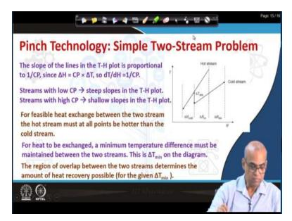
So, what you see now is the temperature enthalpy plot for both the hot stream and the cold stream. Note that it will be a straight line. We are considering that the specific heat does not change between the supply temperature and the target temperature it is a straight line. If the assumption does not hold then of course; it will be a curved line, but then we can always consider that as a piecewise linear segments. And thereby, it will be a series of straight line segments.
