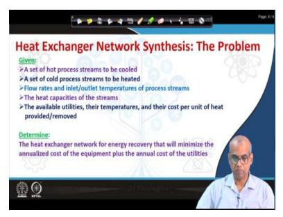
So now let us define formally the problem for heat exchanger network synthesis. We say that given a set of hot process streams to be cooled. A set of cold process streams to be heated. Flow rates and inlet outlet temperatures or process streams, the heat capacities of the streams the availability utilities, they are temperatures and their cost per unit of heat provided or per unit of heat removed.
