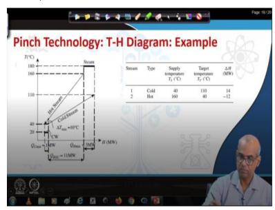
Now let us take an example with some numbers so that we can understand how much of these savings that are possible. So, you have two streams cold stream and hot stream. The cold stream starts with temperature 40. And the target temperature is 110 the hot stream is available at 160
