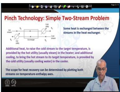
Now, let us take a simple example with only two streams. So, what you see in the figure is there is a hot stream there is a cold stream some amount of heat exchange is taking place between these two streams and also there is additional heat to raise the cold stream to target temperature. And additional cooling to bring the hot stream to it is target temperature. So, there is a hot stream and there is a cold stream they are exchanging heat here in the heat exchanger.
