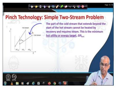
So, this is we just discussed the part of the cold stream that extends beyond the start of the hot stream cannot be heated by the recovery and require steam. So, this is the minimum hot utility or energy target.
