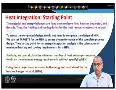
So, where do you start when you do heat integration? As we discussed before the material and energy balances are fixed for a process. Once we have fixed the reactor, the separator and the recycled system. So, during your conceptual synthesis of the flow sheet, once you have fixed the reactor system, the separator and the recycle system you are finalized your material balance and energy balance.
