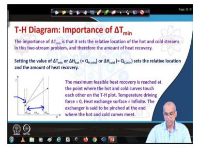
When you set the delta T minimum, it sets the relative position of the hot stream and the cold stream on the T H diagram. And it automatically sets the amount of heat that can be recovered the hot utility target as well as the cold utility target. You will see from the graph that by setting delta T minimum or by setting hot utility target or by setting the cold utility target. The relative position of these two curves on the T H diagram will be fixed.
