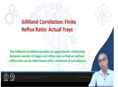
Now after we have found out the minimum number of plates at total reflux condition using the Fenske equation and after finding the minimum reflux ratio using underwood equation will now find out the actual number of trays when you use finite reflux ratio by making use of Gilliland correlation. The Gilliland correlation provides an approximate relationship between number of stages and reflux ratio so that an optimal reflux ratio can be determined with a minimum of calculations.
