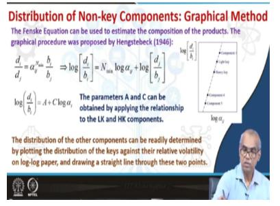
Now finally we will talk about how to determine the distribution of non-key components. It can be done graphically using the Fenske equation. Note the Fenske equation in this form of molar flow rates of distillate and bottoms, you can take logs and can write this way. Note that this can be written as log di by bi equal to A + C log alpha i. The parameters A and C can be obtained by applying the relationship to the light key and heavy key components.
