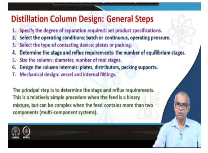
Now, let us first look at the general steps for design of a distillation column. We need to specify the degree of separation required; that means we have to set product specifications. We have to select the operating conditions, first decide on whether it will be a batch process or continuous process decide on operating pressures etcetera. Select the type of conducting devices, are you going to use plate or tray type distillation column or pack type distillation column?
