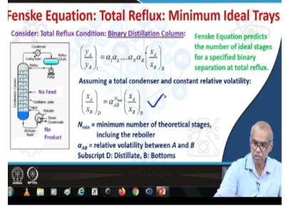
You are perhaps familiar with the Fenske equation for binary distillation columns. The Fenske equation predicts the number of ideal stages for a specified binary separation of total reflux through this equation. Note that if these number of plates, like 1, 2, 3 etcetera up to n, then it is possible to relate the mole fraction of A, divided by mole fraction of B in the vapor around tray 1 with the mole fraction of A and mole fraction of B in the liquid in the bottom through this
