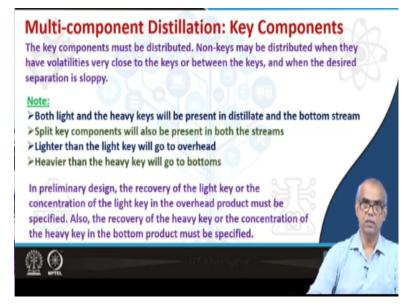
The key components must be distributed. Non-key is maybe distributed when they have volatilities very close to the keys or between the keys and when the desired separation is sloppy, so for sloppy split. Let us summarize, both light and the heavy keys will be present in distillate and the bottom stream. Split key components will also be present in both the streams. Lighter than the light key will go to overhead. Heavier than the heavy key will go to bottoms.
