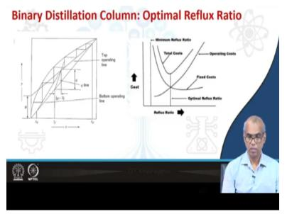
So you are familiar with determination of this number of trays by drawing the steps within the space available between the equilibrium curves and the operating lines for the rectifying sections and the stripping sections. And then finally you are also familiar with the determination of the
