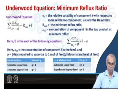
The under root equation is written as this, alpha i x iD divided by alpha - theta, we have to take the sum, this is equal to minimum R reflux ratio + 1. So alpha i is the relative volatility of component i with respect to some reference component, which is usually the heavy key or minimum is the minimum reflux ratio and x iD is the concentration of component i in the top product or distillate at minimum reflux condition.
