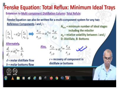
So to use the Fenske equation for a multi component system, we must choose two reference components i and j. Note that for a binary mixture, it was written between components A and B. Now when you have a multi components system we can make use of the Fenske equations, but now it has to be written for any two reference components, say i and j from your multi component system. So this x A by x B in distillate can be written as xi D by x jD or x i by x j in the distillate.
