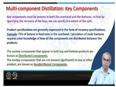
Key components must be present in both the overhead and bottoms, so that by specifying the recovery of the keys, we can specify the extent of the split. Product specifications are generally expressed in the form of recovery specifications. For example, we specify the 75% of butane in feed exists in the overhead. Calculations of mole fractions require prior knowledge of how all the components are distributed between the products.
