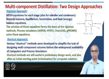
There are broadly two design approaches for multi component distillation columns; one is rigorous approach another is short cut approach. Look at these diagrams, let us say this represents the nth tray in the distillation column. So what you see is all the streams that may be around the nth distillation column, liquid stream, vapor steam, may be the feed stream, may be the side stream and also represents the native flow.
