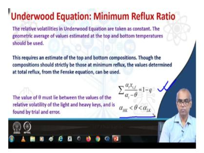
The relative volatilities in underwood equations are taken as constant. The geometric average of values estimated at the top and bottom temperature should be used. This will require an estimation of the top and bottom compositions. Though the compositions should strictly be those at minimum reflux conditions as an approximation these values can be determined at total reflux using the Fenske equations.
