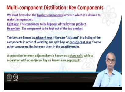
Now, let us understand what do you mean by key components? As you pointed out before for the multi component distillation process, we must first select the two key components between which it is desired to make the separation. These two key components are known as light key and heavy key. Light key, the components to be kept out of the bottom product. The light key is the component which must be kept out of the bottom product and the heavy key is the component to be kept out of the top product.
