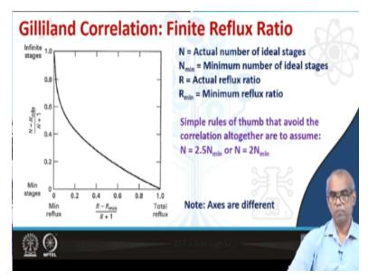
This is the same plot but note that the axes are different. A simple thumb rule which will avoid the correlation altogether is that you can assume the actual number of plates is 2 times or 2.5 times the minimum number of plates, but that is the rule of thumb. We can always make use of this Gilliland correlation to get a better estimate.
