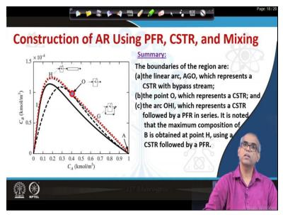
So this is the summary we start with we can start with the PFR the look at the CSTR whether this expense the region or not draw the linear herbs and then find out the scope for further extending that enable region using PFR trajectory, where no further expansion is possible, either through PFR at trajectory or through mixing you have obtained your attainable region.
