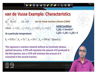
So we will use the shown liquid phase, constant density, isothermal reaction network to illustrate that Attainable Region approach. The reaction scheme known as van de Vusse reaction scheme is basically parallel decomposition of species A. So this represents a reversible reaction. The rate expressions are given. The values of the k1, k2, k3 all the rate coefficients are given at a particular temperature.
