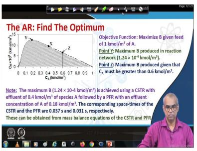
Now let us look at optimization part of it my objective is to maximize B given feed of 1 kilo mole per meter cube of a in this particular case. Clearly from the figure we see that point Y represents maximum B produced in the reaction network. Now if I ask the following question what will be the maximum amount of B produced given that CA must be greater than 0.6 kilo mole per meter cube. So 0.6 is the bound on concentration of A.
