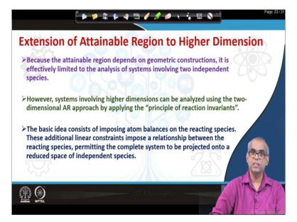
So we will stop this discussion with the comment on how to apply this on higher dimension because the attainable region depends on geometric constructions, it is effectively limited to the analysis of systems involving two independent species. However systems involving higher dimensions can be analyzed using the two dimensional attainable region approach by applying the principle of reaction invariance.
