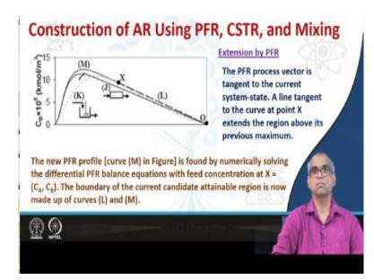
Now let us see whether we can further extend the region by PFR trajectory. The PFR process vector is tangent to the current system step. So a line tangent to the curve at point X extends the region above its previous maximum. Note that this was the previous Trajectory. Now from point X if I draw another PFR trajectory it extends the region above the previous maximum. This is possible because PFR process vector is tangent to the current system state at X.
