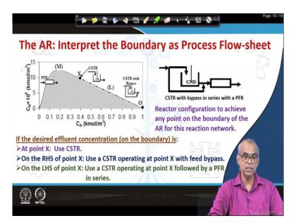
So we can extend the CSTR trajectory by mixing. So again consider the two trajectories the one represented by continuous line is from PFR which is given name J here and this boundary represented by K is CSTR locus. So consider the CSTR locus K, the straight line are OX correcting point X with the feed point O represents the mixing line and these extends the region. So L, line L represents this mixing.
