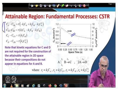
Now let us move on to the next fundamental process CSTR. Again we need to worry only about equations for A and B. Because the kinetic equations for C and D are not required for the construction of the attainable region into this space, because they are compositions do not appear in the equations for A and B. So focus your attention only on first two equations. Note that these are algebraic equations.
