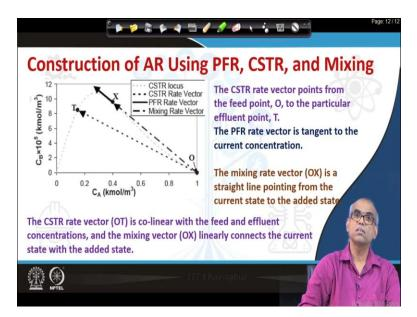
So we will look at the possibility of extending region by not only the mixing process but also by application of PFR trajectory. Now in this figure the CSTR rate vectors are shown as OT which points from the fit point O to a given effluent point T. Note that this dotted trajectory represents a CSTR locus. So point T represents an effluent stream coming out of a CSTR, O represents feed point.
