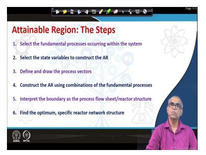
Now, these are the basic states that will follow to construct that enable region. First is we select the fundamental processes occurring within the system. We already said that the fundamental processes that will consider here a reaction and mixing. Select the state variables to construct that Attainable Region. Define and draw the process vectors. Construct that Attainable region using combinations of the fundamental processes.
