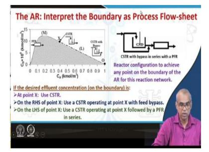
So the construction of attainable region is complete once it has been determined that no other processes can extend the region. The shaded region in the figure shows the entire attainable region for this particular reaction network, that means that van de Vusse reaction scheme. So the boundary of that attainable region is made up of curves L and M. Note that the region is convex it is clear that the mixing cannot extend the region.
