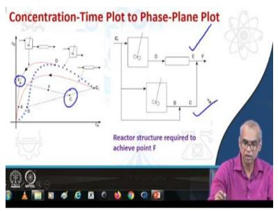
Finally to obtain point F, I have to make point C and point E. Point E is lying on this trajectory which can be obtained by CSTR followed by PFR in series. So you obtain that point E first and then point C can be obtained by CSTR with bypass, CSTR and the bypass to mix the effluent with the feed stream. So this together they will give you point F. So all you have to do is you have to first get E and then you get C with CSTR and bypass and then there being mixed to obtain point F.
