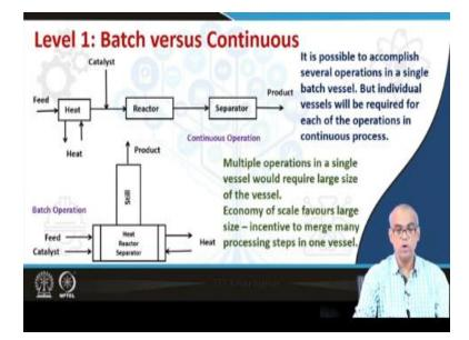
It is possible to accomplish several operations in a batch vessel, but individual vessels will be required for each of the operations in continuous process. Look at the flow sheet for the continuous operation. The equipment that you see, reactors, separators etcetera will be required for individual operations. Whereas for a batch operation the reboiler that you see can be used to supply heat, it can perform the role of reactor, it can also perform the role of separator.
