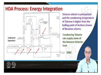
Now the toluene column is pressurized and the condensing temperature of toluene is higher than the boiling point of bottom stream of benzene column. If that is the case, then the condensing toluene can supply some of the benzene reboiler load. So what we just saw is some amount of energy integration in the process.
