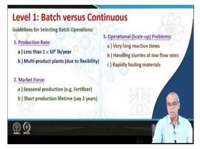
Now, there are certain guidelines for selecting batch operations. So these are the heuristics available which will give you as design guidelines, which will be used as design guidelines to figure out whether we should go for a batch operation or continuous operation. The decisions are based on production rates. If the production rate is less than 1 into 10 to the power 6 pound per year, we go for batch process. Multi product plants due to flexibility will be batch operations.
