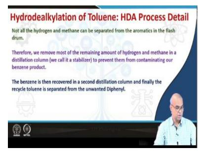
Not all the hydrogen and methane can be separated from the aromatics in the flash drum because it is never a 100% stream. Therefore, we remove most of the remaining amount of hydrogen and methane in a distillation column; we will call it a stabilizer, to prevent them from contaminating our desired product that is benzene. The benzene is then recovered in a second distillation column and finally recycle toluene is separated from the unwanted diphenyl.
