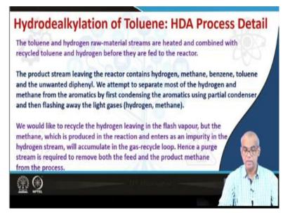
The toluene and hydrogen raw material streams are heated and combined with recycled toluene and hydrogen before they are fed to the reactor. So let us first quickly go through the details of HDA process and then on the basis of this description will try to come up with an intuitive flow sheet for the process. So first the toluene and hydrogen row material streams are heated and combined with recycle toluene and hydrogen before they are fed to the reactor.
