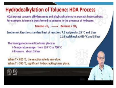
So let us now talk about Hydrodealkylation of Toluene: HDA. HDA process converts alkylbenzenes and alkyl naphthalenes to aromatic hydrocarbons. For example, toluene is transformed to benzene in the presence of hydrogen. So toluene reacts with hydrogen to produce benzene and methane. So we consider toluene, we had hydrogen, this CH3 goes and you get benzene + methane. This is an exothermic reaction. The standard heat of reaction is 7.6. kilocalorie per mole at 25 degree celsius and 1 bar.
