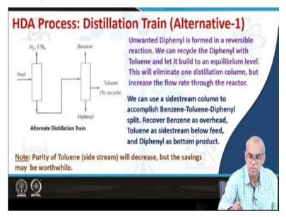
Now, let us focus our attention on the distillation train. Unwanted diphenyl is formed in a reversible reaction. We could recycle the diphenyl with toluene and let it to build to an equilibrium level. This was possible because unwanted diphenyl is formed in a reversible reaction. So this is possible that we can recycle diphenyl with toluene and let it build to an equilibrium level. If we do that, it will eliminate one distillation column, but will increase the flow rate through the reactor.
