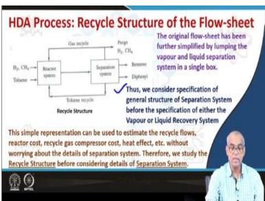
We can further simplify the process flow sheet by lumping the vapour and liquid separation system in a single box. In the previous one, you see we had one box for liquid separation system
