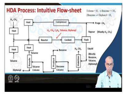
Now on the basis of this, let us develop an intuitive flow sheet. So hydrogen and methane are heated, also toluene which is a liquid under a normal condition is heated to vaporize and also heated to raise the temperature. Then these are mixed and fed to the reactor. So the reactor's stream, the stream that comes out from the reactor, reactor effluence stream will contain the
