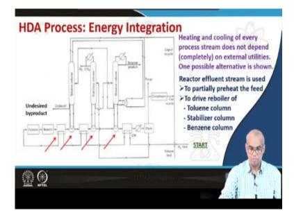
Now, the flow sheet that we just discussed is definitely not an efficient flow sheet because heating and cooling of every process stream depends on external utilities. Now, an efficient flow sheet or efficient process will try to recover waste heat from the process. So it will try to perform energy integration where heating and cooling of every process stream will not depend, at least completely on external utilities. One such possibility is shown on the screen.
