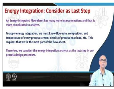
But you could also realize that the flow sheet which involves energy integration has many more interconnections and thus is more complicated to analyze. To apply energy integration, we must know flow rate, composition and temperature of every process stream. We should also note details of process heat load. This requires that we fix most part of the flow sheet. Therefore, it is quite natural that we consider the energy integration analysis as the last step in our process
