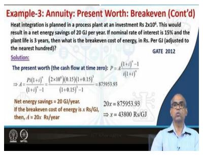
So this is the expression for present worth that means cash flow at time 0 for A uniform series cash flow diagram from this you compute once you compute A equate A to 20 x and then find out the value of x's 43800 rupees per gigajoule.
