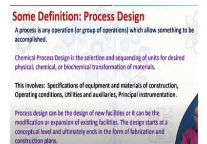
Let us now introduce some definitions. Process design. A process is any operation or group of operations which allows something to be accomplished. Chemical process design is the selection and sequencing of units for desired physical, chemical or biochemical transformation of materials.
