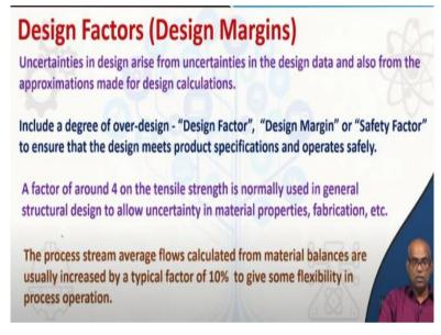
Now when you design a process, uncertainties in design arise from uncertainties in the design data that you use and also from the approximations that you make during design calculations. So to account for this, we have to include a degree of over design which you call design factor or design margin or safety factor. This is required so that the design meets product specifications and operate safely as initially conceived.
