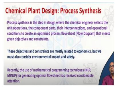
Next, we introduce the definition for process synthesis. Process synthesis is the step in design where the chemical engineer selects the unit operations, the component parts, their interconnections and operational conditions to create an optimized process flow sheet or flow diagram that meets given objectives and constraints. By flow sheet or flow diagram, we mean a diagrammatic representation of the chemical engineering process.
