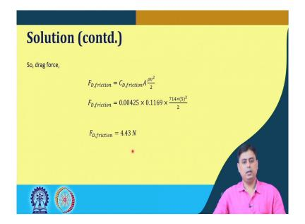
$2\pi rh$  is the available area on which drag force is being exerted and we replace now the numerical values to get the drag force. This skin drag force for the friction drag force over a single tube; so, this is how we calculate drag force, the drag coefficient and related question we have to solve.
