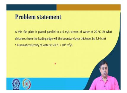
Now, let us quickly have a look at different problem. So, the problem says that a thin flat plate is placed parallel to a 6 m/s stream of water at 20 °C. At what distance x from the leading edge will the boundary layer thickness be of 2.54 cm or 1 inch. So, this is the
