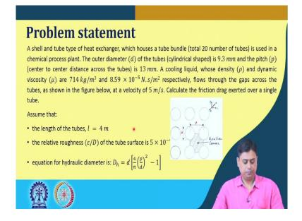
Now, we move on to the third problem. So, here what we see that a problem says that a shell and tube type heat exchanger which houses a tube bundle around 20 tubes in number in a process plant. We use such cylinder heat exchanger in process chemical process plants. So, where these tubes have a outer diameter that is cylindrical in shape is of 9.3 mm and the pitch that is a centre to centre distance during the staking of these tubes.
