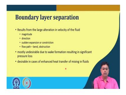
So, this results this boundary layer separation can be resulted from the large alteration of the velocity in the fluid. And, that can be occurred by changing magnitude of the flow field, change in direction of the flow field, it can happen due to sudden expansion or constriction of the flow path, as well as the flow path can be tweaked by bend obstruction or something like that ok.
