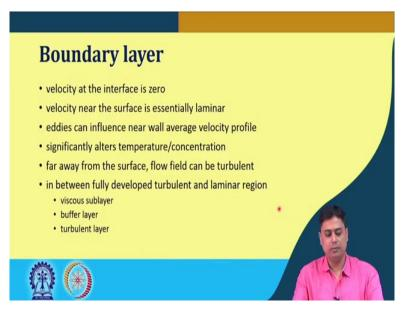
Now, what is fully developed, we will come to that. So, in boundary layer or within the boundary layer there are a few points that you need to remember, that the velocity at the interface or the solid fluid interface is 0, velocity near the surface is essentially laminar, it is of very low velocity flow.
