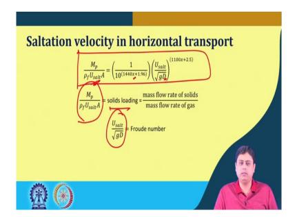
Now, similar to this choking velocity calculation in the vertical transport, there are several correlations for the saltation velocity. Now, in the saltation velocity case as we have seen in the case of choking velocity, if we increase the solids concentration further the saltation velocity also increases from  $G_1$  to  $G_2$ ; that means,  $G_2 > G_1$ .
