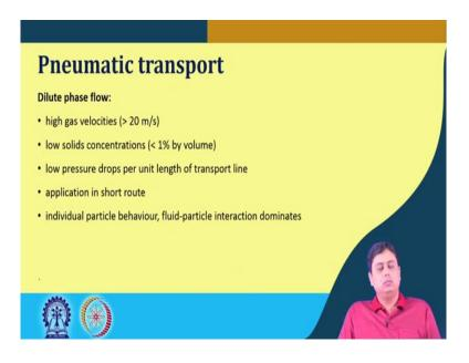
Now, if we go into the details of the dilute phase flow or the transport and the difference between the dense phase transport these two are basically characterized by certain parameters or classified by certain parameters. This can be detected by looking at the gas velocities immediately.
