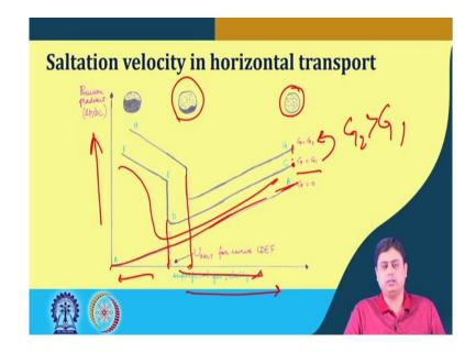
Now, similar to the vertical arrangement in the horizontal transport we can have saltation velocity. Now, here at a very high velocity this is the superficial gas velocity and this is y axis is the pressure gradient. I mean this case again at a very high velocity; we can see that the pipeline cross section is uniformly distributed with the solid particles which is we can say the concentration is lower. So, that this is a dilute phase transport.
