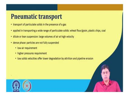
So, pneumatic transport as I mentioned earlier when the fluid phase that carries this solid particle is the gaseous phase. So, the transport of particulate solids in the presence of a gas is called the pneumatic transport or pneumatic conveying. Now, these are widely applied in transporting a various range of particles, that is say starting from wheat flour, wheat grain, plastic chips or even coal.
