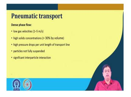
In the contrast in dense phase flow, it can be immediately recognized by the low gas velocities in the range of 1 to 5 m/s, high solids concentration say more than 30 % by volume and high pressure drop per unit length of the transport line. In this case as I mentioned earlier, that the particles are not fully suspended I mean all the particles are not fully suspended.
