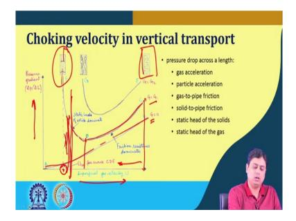
Now, in the case of vertical transport when it is say going against the gravity, now in such case the critical velocity where the operation should be maintained we call that as a choking velocity. And, in case of horizontal flow that velocity we mentioned as saltation velocity.
