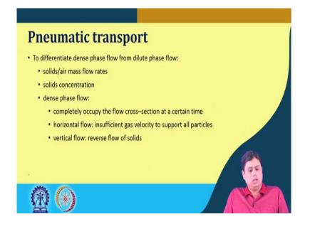
One of such shows or dictates that we can look at these parameters that is listed here, in order to differentiate the dense phase flow from the dilute phase flow. We can look at the solids to air mass flow rates or the ratio. We can look at the solids concentration in the flow, that this helps us in determining which would be the flow regime or which would be the characteristics of the flow.
