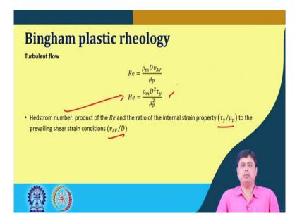
In turbulent flow; which means, we have to again check what is the Reynolds number. Now in this case; this regime transition for the Bingham plastic depends on these two dimensionless number. One is the Reynolds number as well as the Hedstrom number which is *He*.
