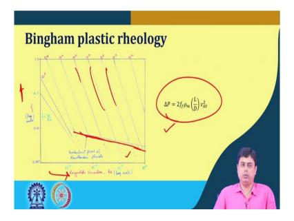
So, quite naturally we have to have a flow design chart, now in this case this flow design the friction factor chart is dependent on the Reynolds number as well as the Hedstrom number. So, these are the Hedstrom number lines and the x axis is the Reynolds number, y axis is a friction factor both are in log log scale, we know this expression for calculation of  $\Delta P$
