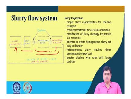
So, if we now briefly look into the other components in the slurry transport that is what would be there in a slurry flow system. So, we basically started with the concept of slurry its different types of slurries that is homogeneous, heterogeneous and in case of salutation design which is not desirable. We have not looked into that because that is not our desirable flow design in a slurry transport, we must avoid that kind of a design at least if it happens in heterogeneous design.
