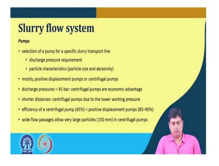
Now, the pump selection, so once slurry is prepared for effective transport we have to choose appropriate pump that can take that to the desired distance. So, since selection of pump for a specific slurry transport line depends on two factors, one is the discharge pressure gradient requirement and the particle characteristics that is its size abrasivity etcetera.
