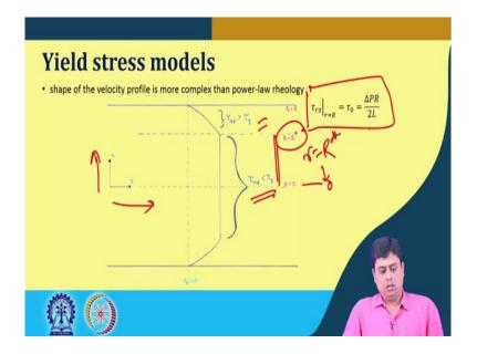
Now, this shape of the velocity profile in this yield stress models is not simple as it was in the case of power law rheology. So, here this is a schematic it shows a typical velocity profile when it flows through a horizontal pipe. So, this is our actual direction this is the radial direction. And we see that, there is a zone of  $R^*$  to the radius, the radial distance is 0. In this zone; we see there is a flat velocity profile. The gradient of the velocity in this direction is 0.
