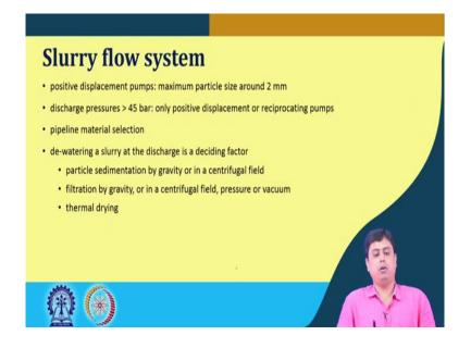
On the contrary positive displacement pump can handle a maximum particle size of 2 mm. So, you already have a selection criteria there, if this discharge pressure is also greater than 45 bars. Then only positive displacement of the reciprocating pumps can be used that is technically feasible.
