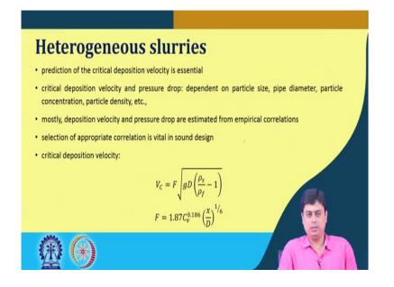
Now, this was the discussion on the homogeneous slurries that is we thought or we assumed that the particles are not settling it is suspended till the flow all the flow happens or the slurry flows from one place to other place. But, in case of heterogeneous slurries we know its nature that few particles will tend to settle, but it will settle in the saltation regime.
