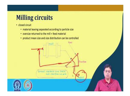
In case of closed circuit operation the materials leaves the milling operation or the grinding operation and then it is separated according to the particle size and over size particles again fed back to the inlet along with the fresh feed. So, it is a kind of a closed loop scenario.
