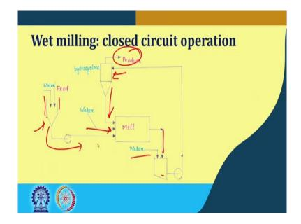
In case of wet milling and again closed-circuit operation because as I mention closed circuit operation is more popular because of its efficiency.
