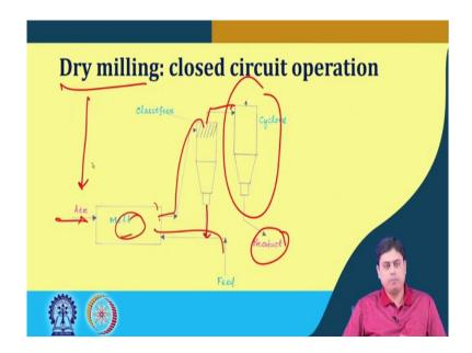
So, the other operations that you mentioned can be of dry or the wet. So, dry milling in absence of any water, most popular liquid phase in the wet operation is the water. So, here what happens in dry milling either air or some other gaseous carrier medium is used it takes the feed to the mill.
