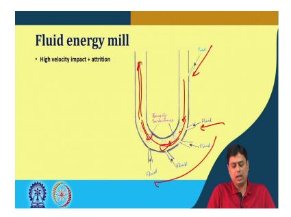
In case of fluid energy meal, here we have very high velocity impact plus attrition. How it works? The feed comes in such cases and then it comes with a very high velocity, the fluids are injected at a very high velocity. So, this fluid or the carrier fluid that also carries the feed, as it comes with a very high velocity it creates zones of turbulences. Now, as it happens the particles are falling and it is being hit by the jets of this fluids which means a very high impact.
