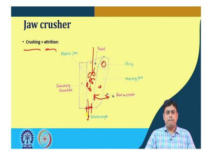
So, for example, if we look at the jaw crusher what happens here is that we have a static jaw there are two solid surfaces in which one is fixed, the other one is hinged at the top up side and this has a jaw action which crushes the particles when the particles are fed from top and discharged through the bottom. So, it is a moving jaw and this is a static jaw. So, it presses against the static jaw and the solid particles are crushed.
