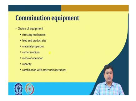
A brief overview of the equipments, that are typically used in a classical size reduction process. Now, the choice of this comminution equipment depends on the stressing mechanism. This we elaborately have discussed. We have also mentioned that what is the size reduction ratio that you are looking at it that what is the feed size and the product size. Based on that, we have to choose the appropriate or suitable equipment.
