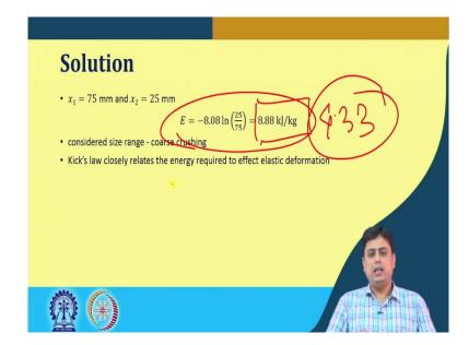
Using this Kick's law constant and for  $x_1=75$  mm and  $x_2=25$  mm we can find the energy requirement which is 8.88 kilo joule per kg. So, from Kick's law it says we have a energy requirement of this much 8.88.
