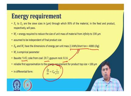
So, this top size, how do we define top size; it is not easy to measure top size. So, this is  $X_1$  and  $X_2$  are basically the same sizes in micron through which 80% of the material in the feed and the product respectively can pass. And this law particularly has stressed on this 80% of the material to be passed passing through and  $W_I$  is the energy required to reduce the particle size of a unit mass of particle from infinity to 100 micron.
