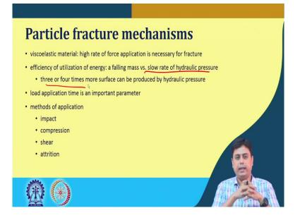
So; that means, an interesting comparison say, you have a falling mass and there is a slow rate of hydraulic pressure that is impacting a certain material in which case, you would expect that the more surface should be created. It is the latter one that is the slow rate of hydraulic pressure; it can create even three to four times more surface which could be produced by a single fall of a mask on that object.
