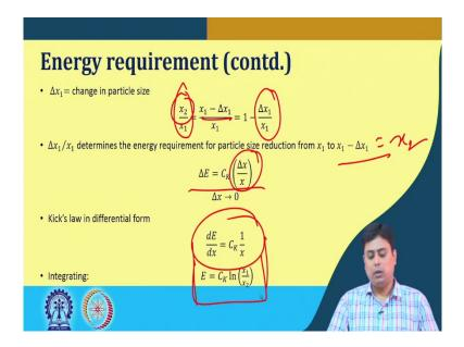
So, if  $\Delta x_1$  say the change in particle size so; that means, x 2 is nothing, but  $x_1 - \Delta x_1$ . So, this size ratio is basically the  $\frac{\Delta x_1}{x_1}$ ; this is what influences the size ratio. The change in particle size with respect to the original particle size, it determines the energy requirement for particle size reduction from  $x_1$  to  $x_1 - \Delta x_1$  which we considered as  $x_2$ .
