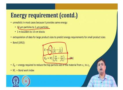
But that does not happen say from  $10 \,\mu m$  particles to  $1 \,\mu m$  particle the amount of energy that would be required and from  $1 \,m$  boulder to  $10 \,cm$  block, this is not the same amount of energy that would be required. So, the point is that the range of experiments or the range of data that
