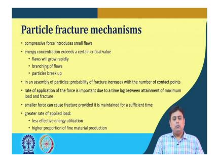
So, this compressive force introduces small flaws and the energy concentration; if it increases or exceeds beyond a certain value, then the flaws will grow rapidly, it branches and the particles breakup. And in assembly of particles, the probability of this fracture increases with the number of contact points between the particles. When the rate of application of this force is another important parameter because the time lag between the attainment of maximum load and the fracture exist.
