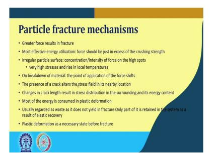
And in particular, we were on the particle fracture mechanisms. So, we have now understood that the ways of particle fracture that can be introduced. So, there was a there is a elastic limit and we have to come across that elastic limit to introduce the fact fracture. Due to the irregular surface in realistic cases, the applied force or the intensity has its stress distribution on the surface of the solid particle.
