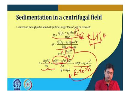
So, which means this  $t_R$ ; then we can write in terms of this Q. So, the Q becomes this V' divided by  $t_R$  which is the expression that we derived.
