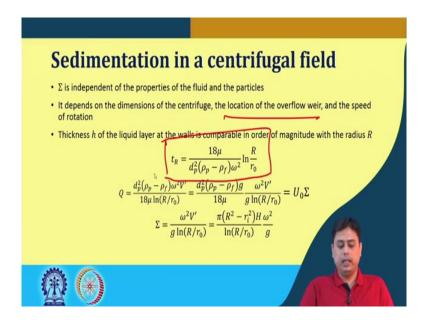
So, this capacity factor is independent of properties of liquid and the particles. It depends on the dimension of the centrifuge, the location of the overflow weir and the angular rotation speed. (Refer Slide Time: 24:44)
