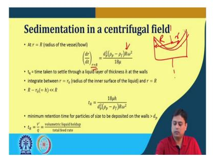
Now, let us say this R as I mentioned the radius of the vessel. So, if this is the vessel, it is rotating on its axis and the free surface takes a form like this. Say particle is here this is R. So, when r is R, it basically the particle hits the wall, impacts a wall. So that means, this expression at R is r. This R is introduced in this place of r.
