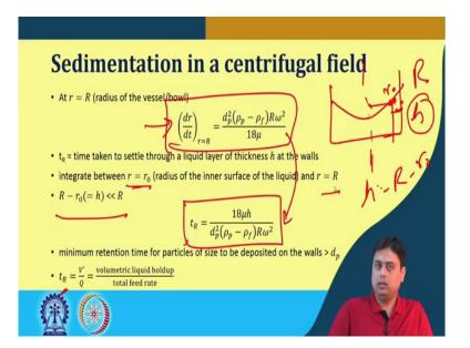
So, we if we now think of a scenario that this is now basically the particle here, if this is my rotating bowl, rotating in this axis and this free surface takes of this form and the particle on this surface is r.
