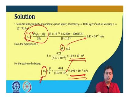
So, we quickly see that the terminal velocity of this 5  $\mu$ m particle because this is the particle size for the first part that is given. We can easily calculate the terminal velocity
