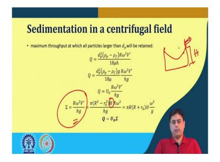
The location of the overflow weir, it indicates this height H; that means, once this fine particle this height H dictates that where the overflow should be going out. So, this is the thing that we can calculate here what is the capacity.
