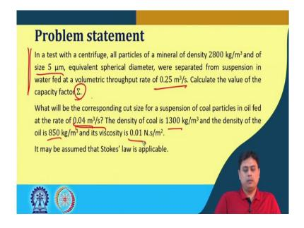
For example, say in a test with a centrifuge all particles of mineral density having 2800 kg/m<sup>3</sup> of size 5  $\mu$ m that is the equivalent sphere diameter, were separated from suspension of a water at a volumetric throughput rate of 0.25 m<sup>3</sup>/s.
