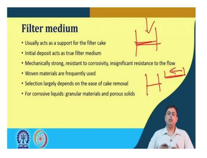
Now, we will move on to the several practices that actually happens during this filtration process that what are the suggested processes or what are the suggested criteria to follow an appropriate filtering condition. The immediate point is the filter medium that you should choose or that is chosen for a certain process. We have to remember that this filter media is basically acting as a support to the filter cake.
