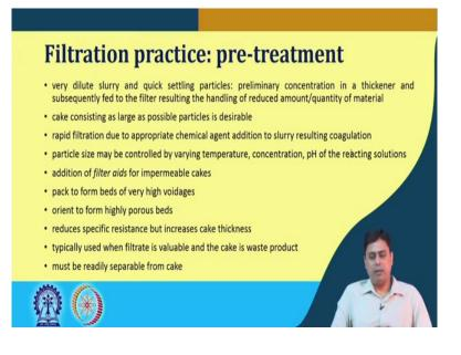
So, we have mentioned there is pretreatment whenever that is required. So, when there is a very dilute slurry and quick settling particles are there, then it is logical and in fact the pretreatment happens in a thickener to concentrate that solution of the suspension, then what happens? You can handle a reduced amount of the slurry.
