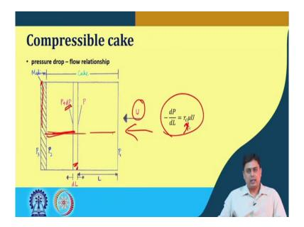
So, how do we deal such system? So, let us say we have a filter medium which is the shaded part. The flow is happening from this right side to the left side. Now, this is happening at a velocity U, we take a let us say this is the thickness of this cake that has been deposited, ok.
