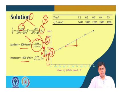
So, basically we find what is  $\frac{t}{V}$ . And then if we plot this, this  $\frac{t}{V}$ , again this is the schematic not to the scale. The point here is that if we have all this points, and this y=mx+c ok. So, which means the gradient would give us this parameter m, and the intercept which is this one the c component.
