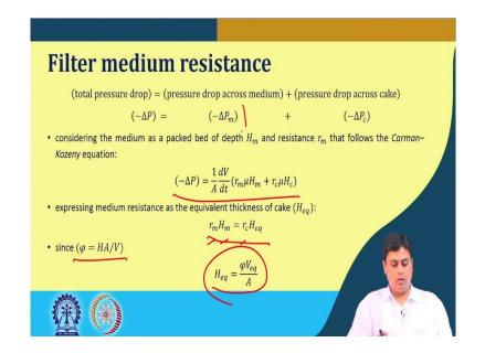
Last time we have seen the relation of the pressure drop with the filtrate volume, without the filter medium resistance as well as including the filter medium resistance. So, this two slide, the initial two slides basically summarizes that what we had concluded last time, that when the filter medium resistance is incorporated in the total resistance, then how the relationship between the pressure drop and the filtered volume was derived.
