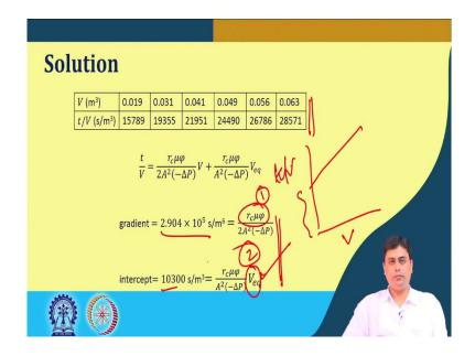
So, which means if we quickly look at the solution the point is that V versus t by V data set is given ok. If we plot this, it would give us, this is the t by V axis in the y-axis, and this is the V. The intercept value would be  $10300 \text{ s/m}^3$  and the gradient would be  $2.904 \times 10^5 \text{ s/m}^6$ . From these two expressions, we find out this two variable which I am marking as 1 and 2 it is not the variable, but the parameters.
