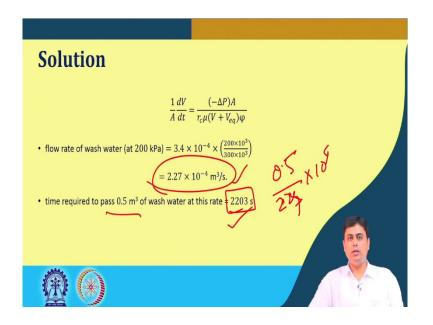
But currently the applied pressure is 200 kPa, which means our wash rate or the filtration rate will be reduced proportionality.
