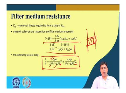
Now, this  $V_{eq}$  and  $H_{eq}$  is the relation is that this  $V_{eq}$  is basically the volume of filtrate that must pass through the filter medium to form a cake height of H equivalent. And this property is only depends on the suspension and filter medium properties. By doing so, we have come
