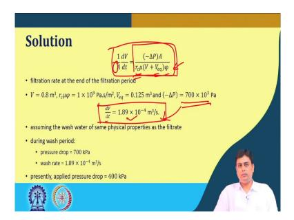
So, now that means, if we now look at the second part, how do we solve we know this is the filtration rate expression. So, this filtration rate expression, and at the end of the filtration experiment, what is the filtration rate. At say, at the end of a filtration rate with this 700 kPa pressure drop and 0.8 m<sup>3</sup> of volumetric flow rate that we have required,
