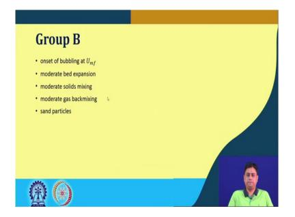
In group B particles at minimum fluidization velocity we have onset of bubbling because, there is no window for the non-bubbling fluidization. We have moderate bed expansion relatively lesser than the group A particles, relatively lesser mixing of solids as well as lesser gas mixing than the group A particles. The example of this group B particles are let us say the sand particles, the building sand particles.
