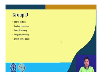
Group D particles are coarser materials or the coarser particles ok; as the size increases it there at a particular or at the same operating condition there is low bed expansion; there is low solids mixing, but better than group C particles. We have low gas backpack mixing; the examples are like gravels, coffee beans and something like that which are bigger in size fine.
