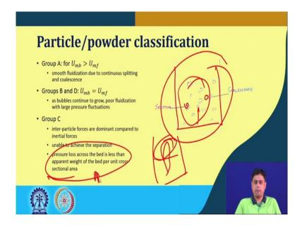
So, if we go into this further this group A material for a condition that is the minimum bubbling velocity when that is higher than the minimum fluidization velocity  $(U_{mb}>U_{mf})$ ok. As we have mentioned that this kind of scenario that happens that in a bed this bubbles forms because, we have reached minimum bubbling velocity. And, then there are coalitions splitting everything is happening continuously throughout the bed and this helps in having smooth fluidization, ok.
