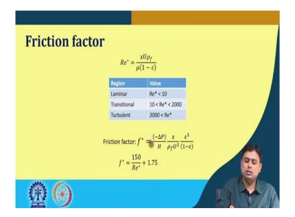
Now the point is friction factor ok. If you remember the friction factor in Fanning friction factor ok, in similar way or analogous to that friction factor, we can define the Ergun equation in terms of the friction factor as well by defining the friction factor as,
