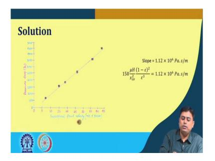
So, we do that, we see that the superficial fluid velocity and the pressure drop. These are the points which we can fit through a straight line with a slope of  $1.12 \times 10^6 Pa.s/m$ . That establishes the flow or the operation is happening in the laminar region. I hope this concept is clear that if we plot the  $\Delta P$  versus U data; the superficial data and if it becomes a linear, then undoubtedly we can say this operation is happening in laminar region for a single phase case.
