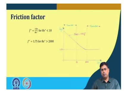
And in case of in case of turbulent the friction factor value is a constant which is 1.75 eventually this friction factor and the  $\Re_p$  in a log scale would look like and this way that it
