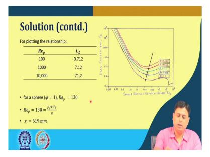
So, here we see that standard drag curves will have these many lines that this we have already discussed in the previous class that with the changing its sphericity this line shifts upward as it goes away from 1 typically it all the values are lesser than 1, then it shifts upward ok.
