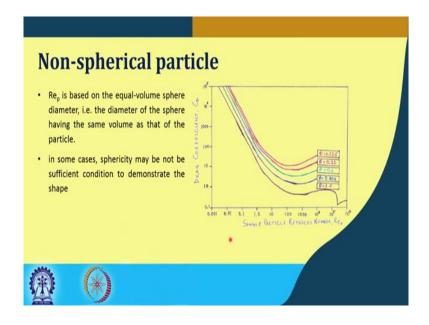
So, typically again like the other cases; this is typically quantified by such plots or the tables that are given, where the particle Reynolds number in this non spherical object are based on the equal volumes sphere diameter ok. Because here you can understand when it is settling or rising; it is the displacement volume or the buoyancy force that becomes one of the determining force ok. So, it is the volume the equivalent volume of the sphere is that what matters ok.
