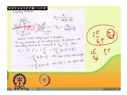
Suppose a fluid let us say oil enters into this phase, I want oil to go into this phase from left to right. So, then in that case since the radius is more, so the capillary pressure would be less right. Here I can see the finally, it is the r m and I can see in this case the r m 2 is more. So, if we talk about 2 sigma divided by r m 2 r m 2 and then this r m 2 is more. So, naturally I have r m 2 is higher when r m 2 is higher the capillary pressure would be less capillary pressure would be less.
