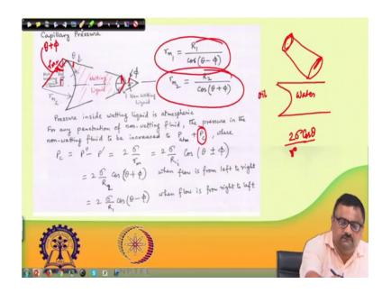
Now, capillary pressure, we said that for a cylindrical system we already said that if you have a cylindrical pore if you have a cylindrical pore and inside it is water the substrate is water wet type; that means, it is like glass and water, the contact angle water mix here is less than 90 degree.
