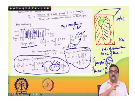
Now, we need to define at this time, what is known as the saturation of a phase saturation of a phase when it comes to flow through porous medium. Now we have two phases, so, I have a void space present say let us say this is a differential volume I have taken out of these this is the solid part and this is the this is the void part. And within this void I can have two different phases, we said water and oil or wetting and non wetting phases.
