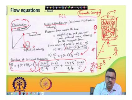
So, what we have here is a process which is known as fluidization; a process which is known as fluidization. What is exactly fluidization? Let us say I have a packed bed and here we have these. So, I have these particles and these are constituting so these are all filled with particles and we are having a flow let us say, we have a flow rate of Q over that overall cross sectional area is let us say E. So, superficial velocity is Q divided by A that is the superficial velocity.
