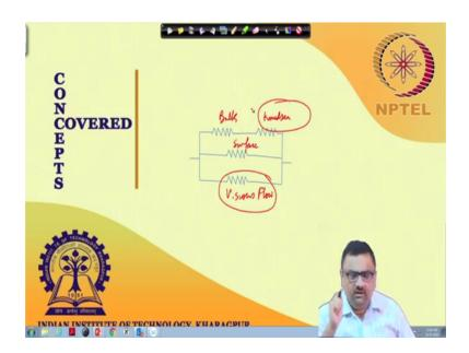
So, in this context what we did is we mentioned that there could be, there could be let us say on one hand we have this viscous flow and this viscous flow is applicable more when we have larger pores. Whereas, there could be a Knudsen diffusion, there could be surface diffusion, there could be bulk diffusion. And then so, there are by various means these transport can also take place.
