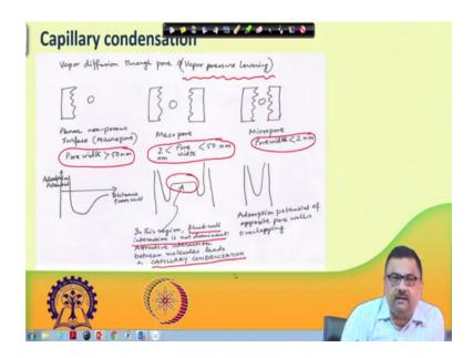
So, here we are talking about vapor diffusion through a pore, and there is a unique thing that happens inside which is known as vapor pressure lowering. So, we will be targeting that. What we have here is we have three different situations presented here, in one case it is planar non-porous surface, these are so called macro pore where pore width is greater than 50 nanometer.
