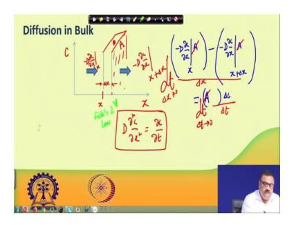
So, now if we if we look at case of say I have a concentration here as a function of x. Now, suppose concentration is flow the diffusion is happening from higher concentration to lower concentration. In that case the flux at this point, flux is minus D del c del x at this location which is let us say x and flux will be; so, this is minus D del c del x at x.
