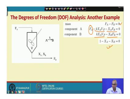
So, number of independent variable is 1, so degree of freedom is 2 minus 1 equal to 1. Final state this example p or a enters to this reactor with volume V, a reaction takes place A to B reaction at constant is k and the outlet stream the flow rate is F R, unit is mass per time and let us say the mole fractions are of A and B are X A and X B in the outlet stream.
