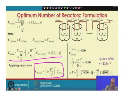
So, now if we apply this recursively we will be able to write CA n out equal to 1 plus kV by Q to the power minus n C A 1 in. What will happen basically is if you use these things recursively, you will be able to write C A 1; note this how this C A n out and C A 1 in are related. This equation needs to be applied recursively.
