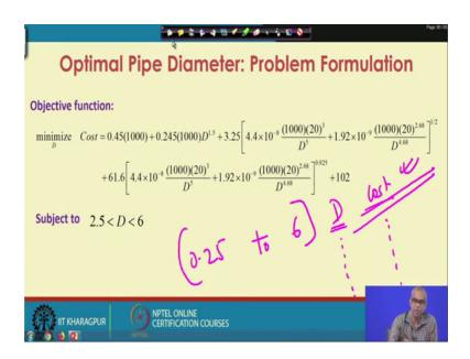
See you basically have an expression for cost versus diameter. So, what you can do is between 0.25 to 6 inch, you can generate the D values and can obtain the corresponding the cost values using this expression.
