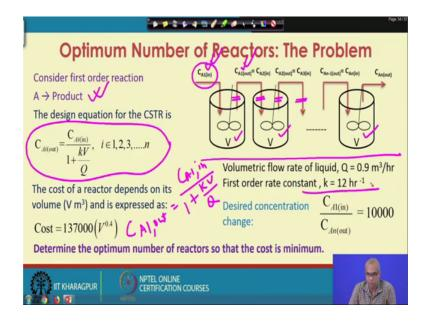
So, let us try to understand the problem first. So, we have n number of CSTR s in series. So, an inlet stream with concentration C A1 in enters CSTR 1. The first order reaction A to products is taking place in each of this CSTR s. So, the outlet concentration of CSTR 1 is the inlet concentration of CSTR 2. The outlet concentration of CSTR 2 is the inlet concentration to CSTR 3 and so on and so forth.
