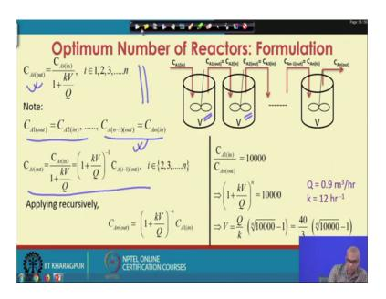
So, this was the design equation C A i out equal to C A i in divided by 1e plus kV by Q; now you understand that the outlet concentration of a CSTR is the inlet concentration to the next CSTR. So, C A 1 out equal to CA 2 in; C A 2 out equal to CA 3 in up to C A n minus 1 out equal to C A in.
