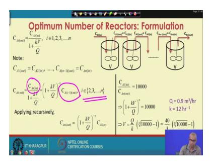
This C A i in is basically C A i minus 1 out. We know that the inlet concentration to a particular reactor number i is basically the outlet concentration of the reactant i minus 1. So, C A i in equal to C A i minus 1 out. Note that this is valid for i equal to 2 3 up to n starting from 2.
