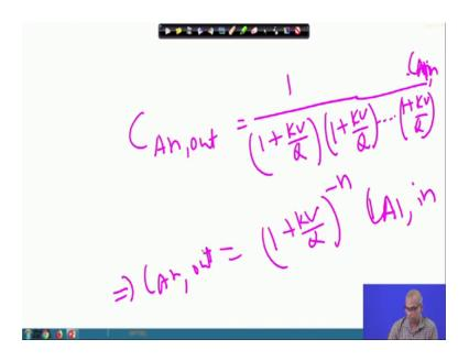
If you do that what will get is C A n out 1 by 1 plus kV by Q 1 plus kV by Q in such term when you have here C A 1 in. So, this leads to 1 plus kV by Q to the power minus n C A 1 in. So, that is what you get this expression.
