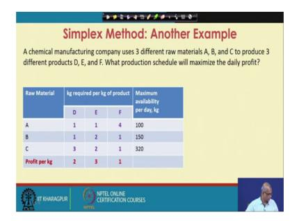
Now, let us take another example. A chemical manufacturing company uses 3 different raw materials A, B and C to produce the different products D, E and F. So, there are 3 different raw materials. Using these 3 different raw materials, 3 different products can be
