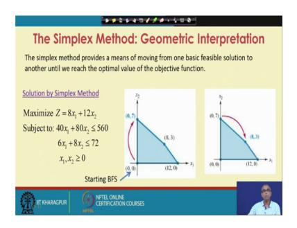
Now, if I solve the same problem using simplex method, I will introduce two slack variables here; S 1 and S 2. So, that the inequality constants become equality constants and S 1 and S 2 will be considered as basic variable x 1 and x 2 will be non basic variables. So, starting basic feasible solution will be x 1 equal to 0, x 2 equal to 0 which is origin.
