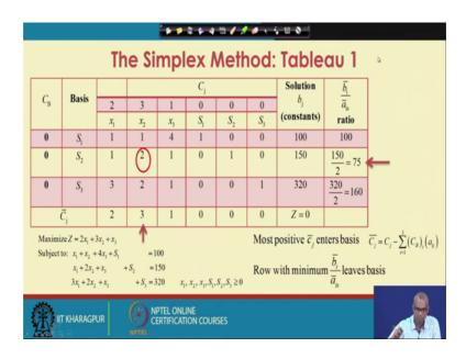
So, this is what you get as Tableau 1. So, S 1, S 2 and S 3 are the basic variables, their cost coefficients are all 0 and x 1, x 2, x 3 are the non basic variables. So, you can check this that is in canonical form and x 1, x 2, x 3 are non basic variables and the coefficients of the constants are written. This column represents the right hand side constants which are 100, 150 and 320.
