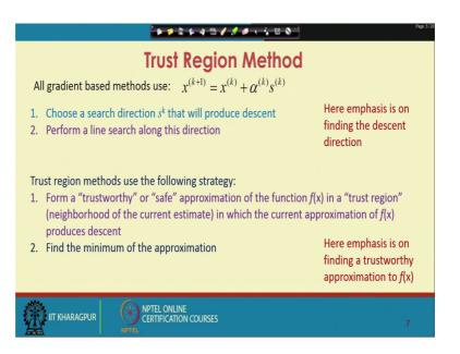
Now, let us briefly define what do you mean by trust region method. We have seen that all gradient based methods use the general scheme x at k plus 1 iteration equal to x at k th iteration plus some stamp step length parameter alpha k into search direction at k. So, in case of gradient based method, we choose a search direction s k that will produce descent. Then perform a line search along this direction Sk.
