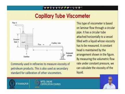
Let us first talk about capillary tube viscometer. The capillary tube viscometer is commonly used in refineries to measure viscosity of petroleum products. This is also used as secondary standard for calibration of other viscometers.
