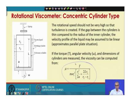
The rotational speed should not be very high. So, that turbulence is created if the gap between the cylinders is thin compared to the radius of the inner cylinder, the velocity profile of the liquid may be assumed to be linear basically it approximates parallel plate situation.
