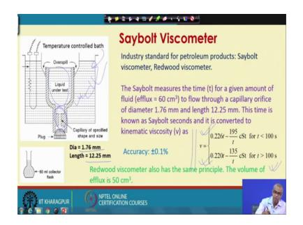
Next let us talk about say bolt viscometer. In fact, say bolt viscometer is an industry standard for petroleum products. Similar to say bolt viscometer there is another viscometer known as redwood viscometer.
