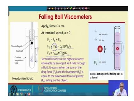
Next, let us talk about falling ball viscometers, falling ball viscometers is another simple setup for measuring viscosity, we are measuring viscosity of Newtonian liquid, here what you do is, you have taken liquid let us say in this tube. Let us consider you have taken a ball let us say made of steel in this liquid you have taken a tube, you have to and you
