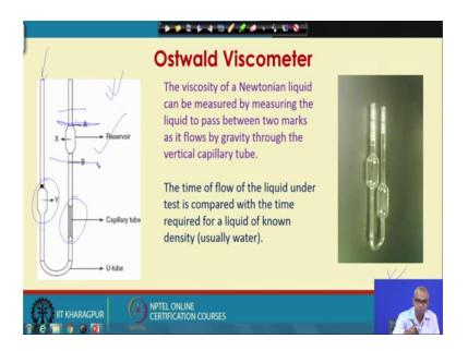
Next we talk about Ostwald viscometer. This is a schematic of an Ostwald viscometer and, this is a real image a photograph of Ostwald viscometer. The viscosity of a Newtonian liquid can be measured by measuring the liquid to pass between 2 marks as it flows by gravity through the vertical capillary tube. So, basically the all viscometer consists of a reservoir, it consists of a capillary tube, it also consists of another bulb layer which can access reservoir.
