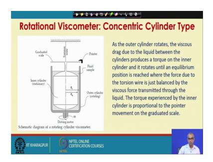
As the outer cylinder rotates the viscous drag due to the liquid between the cylinders produces a torque on the inner cylinder and, it rotates until an equilibrium position is reached, when the force due to the torsion where is just balanced by the viscous force transmitted through the liquid.
