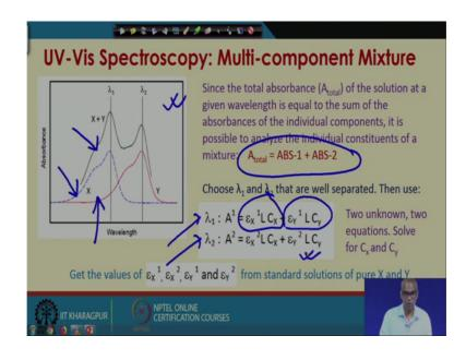
Now, let us say this is the absorption spectra for pure x and this is absorption spectra for pure y. So, when you have a mixture of x and y, you get these as absorption spectra. Since the total absorbance of the solution at a given wavelength is equal to the sum of the absorbance of the individual components. It is possible to analyze the individual constituents of a mixture. Because we know that a absorbed total absorbance is equal to sum of the individual absorbance.
