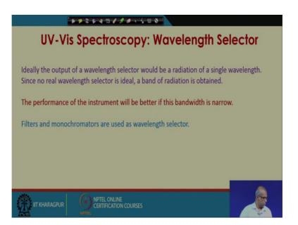
So, wavelength selector is supposed to choose a radiation of single wavelength. So, ideally speaking the output of a wavelength selector would be a radiation of a single wavelength. Since, no real wavelength selected is ideal, a band of radiation is always obtained. The performance of the instrument will be better if this bandwidth is narrow.
