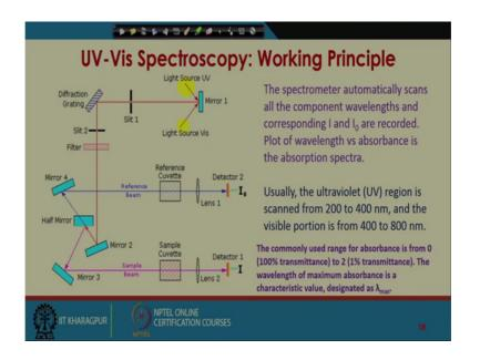
The spectrophotometer automatically scans all the component wavelengths, and corresponding I and I 0 are recorded. From the values of I and I 0, I can find out absorbance and the detector of the UV-Vis spectrophotometer generates a plot of wavelength vs absorbance. This is the absorbance absorption spectra.
