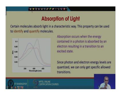
Certain molecules absorb light in a characteristic way. This property can be used to identify and quantify molecules. Absorption occurs when the energy contained in a photon is absorbed by an electron resulting in a transition to an excited state.
