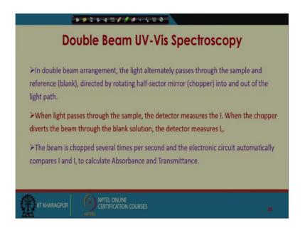
In double beam arrangement the light alternately passes through the sample and reference, directed by rotating half sector mirror or chopper into and out of the light path. When light passes through the sample the detector measures I, when the chopper diverts the beam through the blank solution the detector measures I 0. The beam is chopped several times per second and the electronic circuit automatically compares I and I 0 to calculate absorbance and transmittance.
