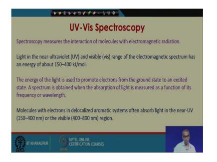
Spectroscopy measures the interaction of molecules with electromagnetic radiation. Light in the near ultraviolet and visible range of the electromagnetic spectrum has an energy of about 150 to 400 kilojoules per mole. The energy of the light is used to promote electrons from the ground state to an excited state. A spectrum is obtained when the absorption of light is measured as a function of it is frequency or wavelength.
