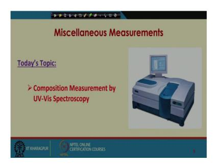
So, todays topic is composition measurement by UV-Vis spectroscopy, and in the screen, you see how a UV-Vis spectrophotometer looks like.
