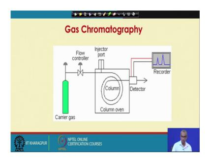
So, these are the various parts of gas chromatography, as we discussed in our previous lecture, you have carrier gas flow controller sample injection system, column you have column oven, detector and finally, the detector gives you the response which is a detector signal versus time graph, which is known as chromatograph.
