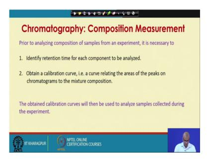
Now, how exactly we measure the composition? Prior to analysing composition of samples from an experiment it is necessary to identify retention time for each component to be analysed and obtain a calibration curve. That is a curve relating the areas of the pigs
