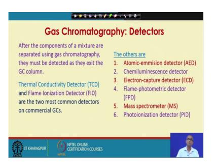
Next, we talk about detectors of gas chromatography. After the components of a mixture are separated using gas chromatography, they must be detected as they exit the gas chromatography column. There are 2 common detectors. Thermal conductivity detector and flame ionization detector are the 2 most common detectors on commercial gas chromatography.
