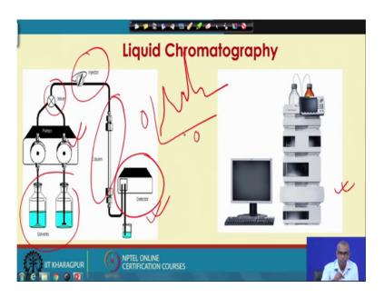
So, this is a schematic of the liquid chromatography, and this is a real photograph. So, you have the solvents, you have the palms. So, they are mixed, you have the sample injection system, you have the column through which the mobile phase is passed at high pressure, and then from the other end of the column the mobile phase or enters the detector which produces a chromatograph, which is detector signal versus time plot.
