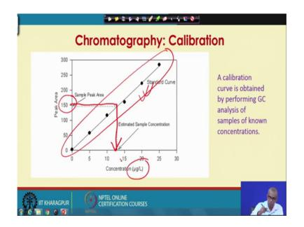
Next step is to obtain a calibration curve. To obtain the calibration curve you have to perform gas chromatographic analysis of samples of known concentration.
