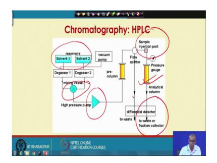
Again, another schematic, you have the reservoirs for the solvents. It is passed to degassers solvents must be degassed, you mix them, you have the high-pressure pump,
