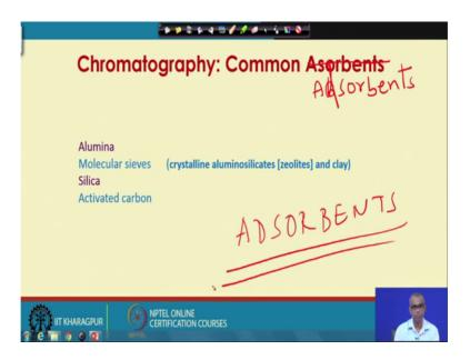
Here some common absorbance, this is absorbance, some common absorbance are or adsorbents, alumina, molecular sieves silica activated carbon. So, alumina molecular sieves this crystalline alumina silicates realized sand clay silica and activated carbons are commonly used adsorbents in the column.
