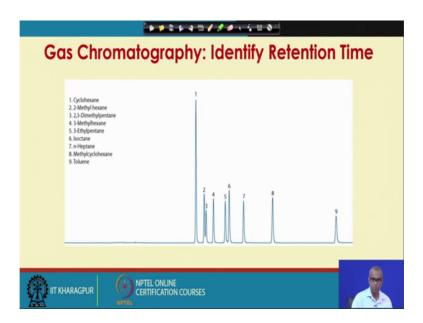
For example, here you have several components. So, you must first perform experiments, with the pure components to know about their retention times. So, then you know that one is pro cyclohexane 2 is for 2 methyl hexane so on and so forth.
