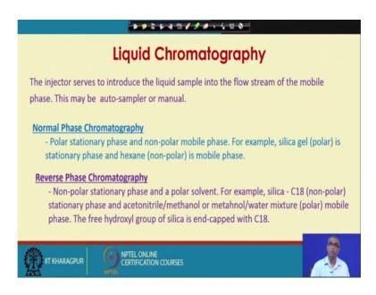
The injector serves to introduce this liquid sample into the flow system of the mobile phase, this may be auto sampler or manual. There are 2 important terminologies one is normal phase chromatography, other is reverse phase chromatography. In case of normal phase chromatography, polar stationary phase and nonpolar mobile phase are used. So, normal phase chromatography means, you have a polar stationary phase and nonpolar mobile phase.
