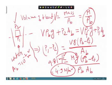
So, volume of the float I can find out because mass is given. So, mass divided by density of the float material let us consider mass as M density is rho b. So, volume of the float is this now what I will do is we will write down the balance equation, the force balance equation upward forces equal to downward forces.
