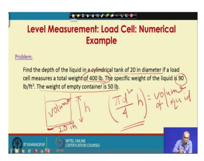
So, let us consider the first problem on level measurement by load cell, find the depth of the liquid in a cylindrical tank of 20 inch diameter if a load cell measures a total weight of 400 pound. The specific weight of the liquid is 90 pound per feet cube the weight of empty container is 50 pound. So, load cell can be used for measurement of level; so,
