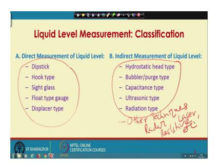
So, if you look at the classification more time these are the instruments that we have covered under direct measurement of liquid level and under indirect measurement of liquid level. We have covered these additionally we have also talked about other techniques of liquid level measurements such as radar, laser based, resistive type etcetera. So, what we plan to do today is we will take some numerical problems on level measuring instrument as well as flow measurements.
