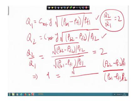
So, if you remember the flow rate expression for rotameter was Q equal to rotameter constant, y the rotameter reading density of the flow minus density of the liquid divided by density of the liquid. So, this was the expression for the flow through rotameter, Now I am using the I am using the rotameter for liquid 1 and liquid 2; so, let us apply this equation for the liquid 1 and liquid 2.
