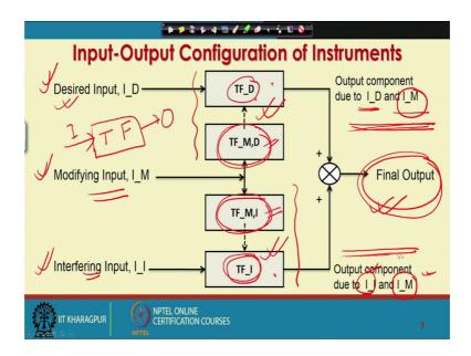
Now, let us see input output configuration of instruments. So, we have now learnt about desired input, modifying input and interfering input, we have also learnt about the transfer function of an instrument. There is a transfer function of an instrument and transfer function works on this input and gives you this output, so this is a mathematical representation for benefit of analysis.
