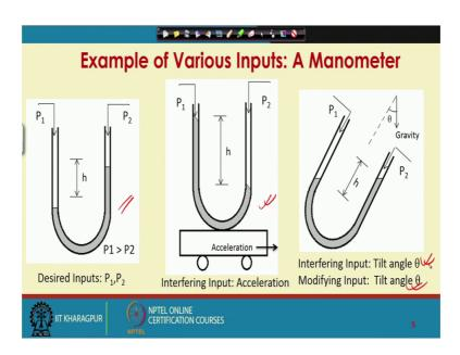
So, what you learn from here is? That for manometer P 1, P 2 the pressure sources in both the limbs get the desired inputs acceleration maybe an interfering input, tilt angle maybe an interfering input, tilt angle can also be an modifying input temperature can also be an modifying input.
