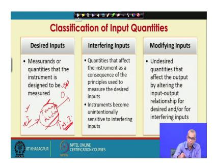
Now, let us classify various inputs that an instrument intentionally or unintentionally receives while it measures a medium a quantity of a medium, desired inputs are those inputs for which the instrument has been specifically design for. So, measured or quantities that the instrument is designed to be measured are desired input, so ideally the instrument should be sensitive only to desired input, because the instrument has been designed specifically for the desired input.
