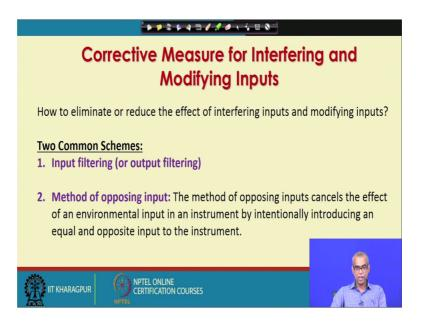
Method of oppose in case of method of opposing inputs we intentionally introduce an input, whose effect is equal and opposite to that of unintentionally sensitive interfering input. So, that it effect so that the introduced input cancels out the effect of interfering input.
