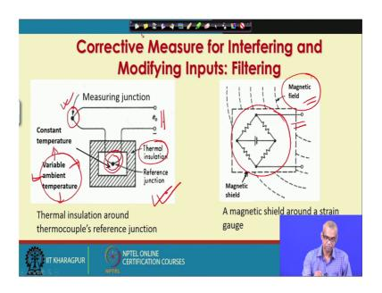
A quick example of filtering this is an example of thermocouple; has two junctions, this is known as measuring junction or out junction, this is known as reference junctions. So, thermocouple made of two dissimilar metals and two junctions are formed, if these two junctions are kept at two different temperatures then this e m f produced will depend on this temperature difference between these two junctions.
