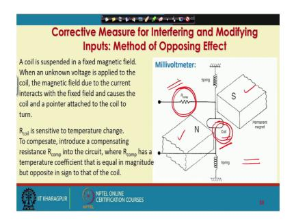
Finally, will take a brief example of method of opposing effect for correcting measure of interfering and modifying inputs; this is an example of millivolt meter, so coil is suspended in a fixed magnetic field, when an unknown voltage is applied to the coil the magnetic field due to the current interacts with the fixed field and causes the coil and pointer attach to the coil to turn.
