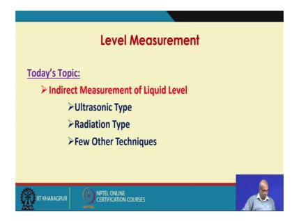
In addition to that we will also talk about few other techniques for measurement of level. So, today we will talk about Ultrasonic Type level gauge, Radiation Type level gauge and briefly we will talk about Few Other Techniques that are used for measurement of level.
