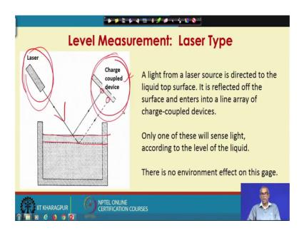
Finally, will talk about level measurement by Laser Type level gauge; A light from a laser source is directed to the liquid top surface. It is reflected off the surface and enters into a line array of charge-coupled devices. So, you have a laser source, you have a charge coupled device which receives the reflected laser beam. Only one of these will sense light. So, there is a line array of charge coupled devices and only one of these will sense light according to the level of the liquid.
