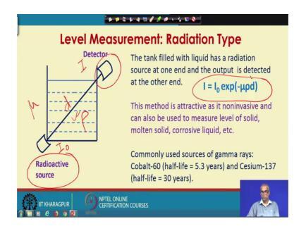
So, on typical design is on in the schematic, we have a Radioactive source. It has been attached at one corner and in the other corner, we have this radiation Detector. So, this Radioactive source emits a radiation with intensity I 0 and let us say the Detector detects the intensity as I. The mass absorption coefficient is mu and the density of this medium is rho.
