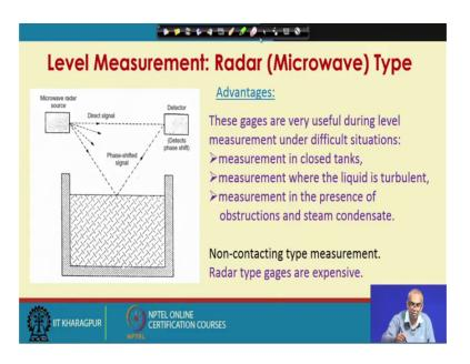
Let us talk about a technique which is similar to Ultrasonic type level measurement. This is Radar Type or Microwave Type. Look at the schematic you have a microwave radar as a source which sense a microwave signal directed towards the top surface of the liquid level and there is a detector which receives the reflected radar signal.
