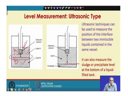
Ultrasonic techniques can be used to measure the position of the interface between two immiscible liquids contained in the same vessel. So, here I have liquid A, I have liquid B. So, liquid A and liquid B are immiscible. So, there is an interface between these two immiscible liquids. So, using ultrasonic device, it is possible to locate this interface between these two.
