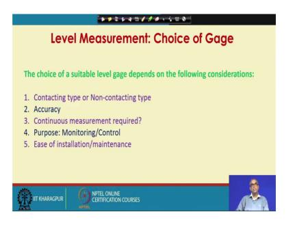
So, finally, we have talked about various level measuring instruments. Now, how do I select a suitable gauge for my application? The choice of a suitable level gauge depends on the following considerations. We must ask whether we need a Contacting type level gauge or Non-contacting type level gauge. What is the accuracy required? Is Continuous measurement required?
