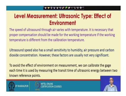
Now, let us talk about Effect of Environment on the measurement of level using ultrasonic type level gauge. As we discussed the speed of ultrasound through air varies
