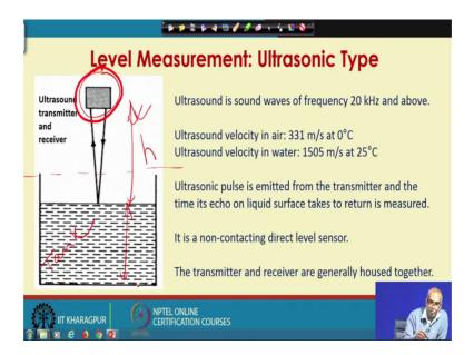
Ultrasound is sound waves of frequency 20 kilohertz and above. The velocity of ultrasound in air is 331 meter per second at 0 degree Celsius; ultrasound velocity in water is 1505 meter per seconds at 25 degree Celsius. So, please note two things; one is
