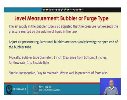
So, the air supply in the bubbler tube is so adjusted that the pressure just exceeds the pressure exerted by the column of the liquid in the tank because when the pressure exerted by the column of the liquid in the tank at the free end of the bubbler tube is equal to the pressure of the purge gas. Then, only the air bubble or nitrogen bubble will escape.
