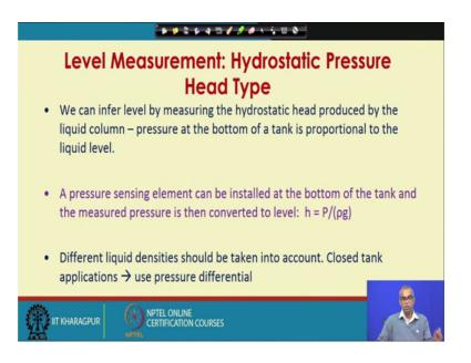
And will start with Hydrostatic Pressure Head Type. We can infer liquid level by measuring the hydrostatic heat produced by the liquid column - pressure at the bottom of a tank is proportional to the liquid level.
