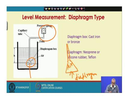
Now, let us talk about Diaphragm type level measurement. What you see in this schematic is a diaphragm in the Diaphragm Box. So, you have this diaphragm you have this gap. So, this is the diaphragm box. So, this is how it looks like here. You have this is diaphragm, this is the diaphragm.
