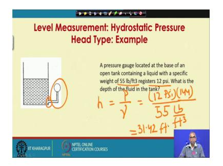
Again, let us take a very simple numerical example. A pressure gauge located at the base of an open tank containing a liquid with a specific weight of 55 pound per feet cube registers; A pressure of 12 psi, 12 pounds per square inch. What is the depth of the liquid in the tank?
