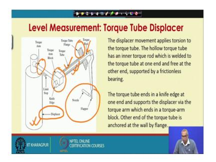
Next to talk about a variation Torque Tube Displacer; In the schematic, this is the Displacer. This is a Torque tube. This is Torque Arm Block. This is Torque Arm and here, I have a Flapper nozzle system connected to one end of the Torque Rod and this part comes out of the wall of the tank and you have this Flange which rigidly connects the Torque Tube with the wall of the tank.
