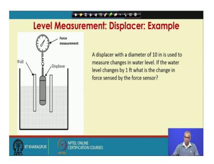
Let us take a very simple numerical example. A displacer with a diameter of 10 inch is used to measure changes in water level. If the water level changes by 1 feet, what is the change in force sensed by the force sensor? So, let us consider this displacer. It is diameter is given as 10 inch.
