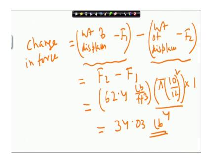
So, change in force will be weight of displacer minus F 1 that is a before, before the liquid level change the 1 feet and this is weight of displacer minus F 2. So, this is this is the force sense by the sensor before changing liquid level and this is the force sensed by the force sensor after the liquid level has changed by 1 feet.
