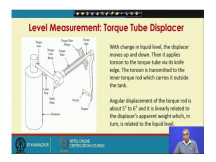
With change in liquid level, the displacer moves up and down. Then, it applies torsion to the torque tube via its knife edge. The torsion is transmitted to the inner torque rod which carries it outside the tank. So, it change in liquid level, the displacer moves up and down. Does it applies torsion to the torque tube via its knife edge?
