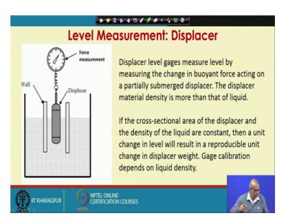
So, we will first start with Displacer type liquid level measurement which comes under direct measurement of liquid level. Displacer level gages measure level by measuring the
