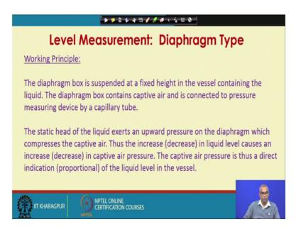
So, to summarize the working principle, the Diaphragm Box is suspended at a fixed height in the vessel containing the liquid. The Diaphragm Box contains captive air and is connected to pressure measuring device by a capillary tube. The static head of the liquid exerts and upward pressure on the diaphragm which compresses the captive air.
