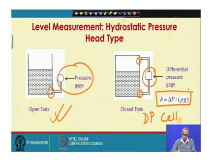
So, hydrated Hydrostatic Pressure Head Type can be used for measuring liquid level in open tank using this pressure gauge attached at the bottom of the tank. I can also measure differential pressure using a differential pressure gauge such as DP Cell by taking a pressure point here and pressure point there and using h equal to delta p by rho g.
