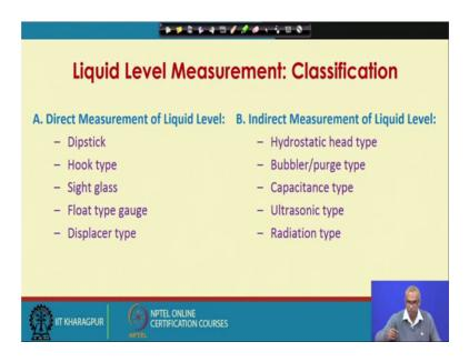
So, this was our classification. So, we talked about Dipstick, Hook type, Sight glass, various Float types including Float and Shaft. So, let us start with Displacer type after
