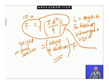
So, I have 10 inch dia displacer. What is the buoyancy force on the cylindrical displacer? Buoyancy force F is pi d square by 4. There is a cross sectional area times L which is the length of the displacer submerged in the liquid. So, L is length of the displacer submerged in liquid and d is the diameter of the float and this has to be multiplied with the specific weight gamma.
