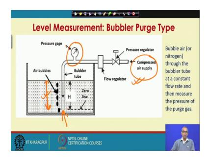
Next, we will talk about a Bubbler or Purge Type liquid level measurement. What you see is a Bubbler or Purge Type level gauge. So, this consists of a Bubbler tube. We have a Bubbler tube. This Bubbler tube has been put to the tank whose liquid level, I want to measure and this is dipped to a certain height. So, let us consider this is dipped up to this.
