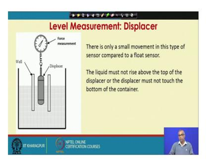
Note that, there is only a small movement in this type of sensor compared to float sensor. The liquid must not rise above the top of the displacer for the displacer must not touch the bottom of the container. So, the displacer will always be partially submerged. (Refer Slide Time: 04:56)
