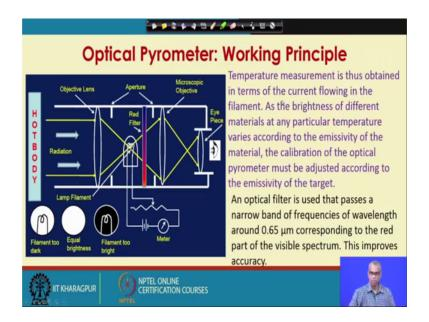
Temperature measurement is thus obtained in terms of the current flowing in the filament as the brightness of different materials at any particular temperature varies according to the emissivity of the material. The calibration of the optical pyrometer must be adjusted according to the emissivity of the target, an optical filter is used that passes and narrowband of frequencies of wavelength around 0.65 micrometer corresponding to the red part of the visible spectrum this improves accuracy.
