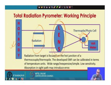
So, this is a schematic of total radiation pyrometer radiation from target is focused on the hot junction of a thermocouple or thermo coil the developed EMF can be calibrated in terms of temperature units wide range it has wide range this is inexpensive and this is simple; however, it is low sensitivity absorption in the of site path may introduced some error.
