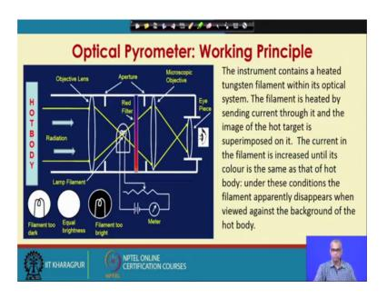
So, the instrument contains a heated tungsten filament within its optical system, the filament is heated by sending current through it at the image of the hot target is superimposed on it by this objective lens. The current in the filament is increased until it is color is the same as that of the hot body under these conditions the filament, apparently, disappears when viewed against the background of the hot body.
