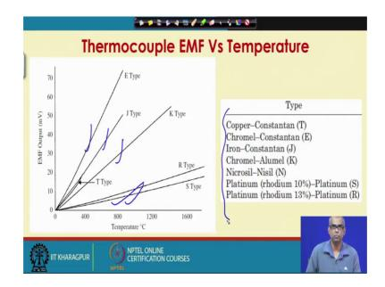
This is a schematic of how the EMF output in millivolt varies with temperatures for different types of thermocouples. You can see in the figure that most of them are approximately linear, not all are linear, but they are approximately linear. So, this is a schematic representation of variation of EMF output in millivolt with respect to temperature expressed in degree Celsius for different types of thermocouples.
