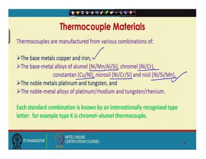
So, now let us talk about thermocouple materials. As of now we have seen what a thermocouple is how to make thermocouple junctions, what are the different junctions, what is Seebeck effect, Peltier effect, Thompson effect, and what are the different thermocouple laws. We have seen all these things in our previous lecture. Now, let us talk about thermocouple materials and different types of thermocouples that are available for measurement of temperature in laboratory or in industries.
