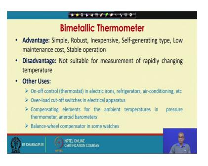
There are some other uses for bimetallic thermometers or bimetallic strips. It is used as on-off controller or thermostat in electric irons, refrigerator, air-conditioning etcetera. It is used as over load cut off switches in electrical apparatus, can be used as compensating elements for the ambient temperatures in pressure thermometer, aneroid barometers. It is also used as balance wheel compensator in some watches.
