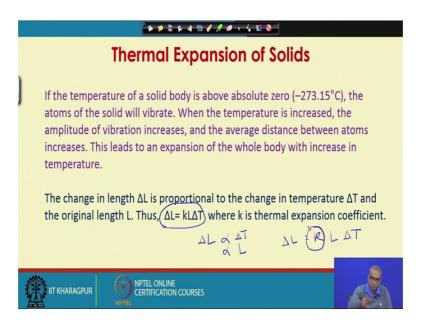
So, we will start our discussion on thermal expansion of solids. Under these, we will be talking about bimetallic thermometer. If the temperature of a solid body is above absolute 0, now you know it is minus 273.15 degree Celsius or 0 degree Kelvin, the atoms of the solid will vibrate, when the temperature is increased the amplitude of
