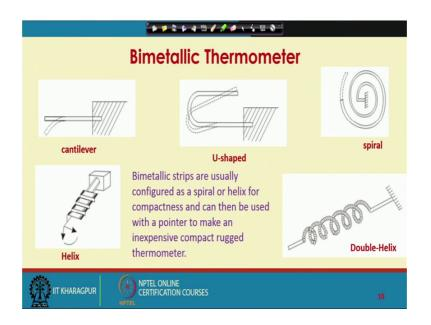
Biometric strips are usually configured as a spiral or helix for compactness and can be used with a pointer to make an inexpensive compact rugged thermometer. So, these are the usual configuration of bimetallic strips, cantilever, U-shaped, spiral, helical and double helix; very commonly spiral and helical configurations are found. In all these cases you see that one end is fixed, and the other end is subjected to the medium whose temperature you are measuring.
