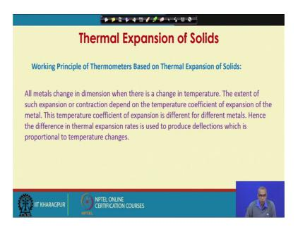
So, following is the working principle of thermometers based on thermal expansion of solids. All metals change in dimension when there is a change in temperature. The extent of such expansion or contraction depend on the temperature coefficient of expansion of the metal. This temperature coefficient of expansion is different for different metals hence the difference in thermal expansion rates is used to produce deflections which is proportional to temperature changes.
