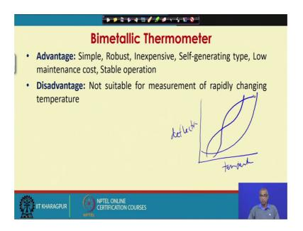
The advantage of bimetallic thermometer is as follows. It is simple, robust, inexpensive, self-generating type; that means, external power source is not require, low maintenance cost and stable operation. Disadvantage; not suitable for measurement of rapidly changing temperature. Also the deflection of different materials typically show non-
