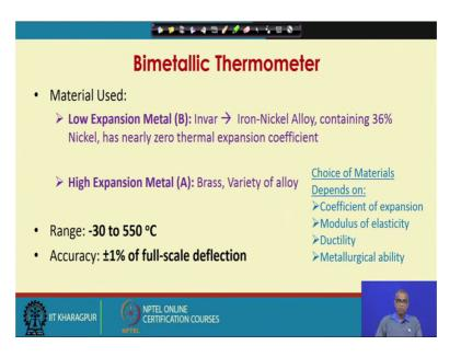
So, what are the different materials that can be chosen for making bimetallic thermometer. Choice of materials will depend on coefficient of expansion coefficient of thermal expansion, modulus of elasticity, ductility, metallurgical ability etcetera. Commonly the low expansion metal B that is used is invar which an iron-nickel alloy containing 36 percent nickel, and has nearly zero thermal expansion coefficient.
