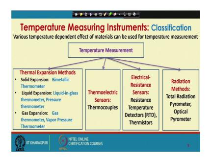
So, how do you classify various temperature measuring instruments? There cannot a single way by which we can do that; there are various temperature measuring instruments; we can classify differently. Let us say we can classify based on their range; we can classify based on whether they are contacting type or non contacting type such has whether it is necessary for the purpose of measurement to bring the instrument in direct contact to the medium whose temperature is measuring.
