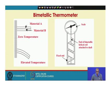
So, this is another example or schematic. You have this bimetallic strip made of material A and material B. One end is fixed. If you take it to a temperature different than the bonding temperature or elevated temperature, it has bend like this. So, this deflection is a measure of the temperature. So, here you see inside, you have a helical coil of bimetallic strip.
