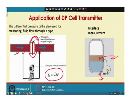
The differential pressure cell can also be used for measurement of fluid flow through a pipe. A fluid is flowing through this pipe. I have put an orifice plate we will learn more about orifice plate or orifice meter when we talk about measurement of flow. For the time being let us consider that the orifice plate works as a flow restrictor. So, we have put
