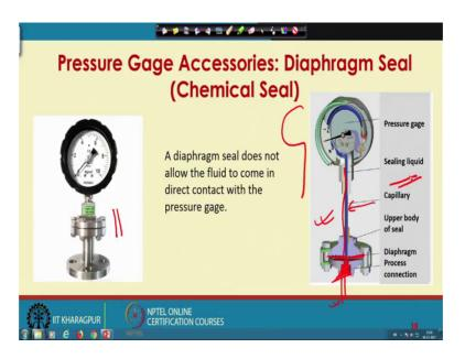
A diaphragm seal does not allow the fluid to come in direct contact with the pressure gage. So, here I have the diaphragm seal also known as chemical seal. So, look at here now, we have a diaphragm; this is the process fluid this is the pressure gage. Let us say this is the bourdon tube pressure gauge and this is the capillary. So, this capillary and the entire bourdon tube is completely filled with the sealing liquid pressure silicon oil.
