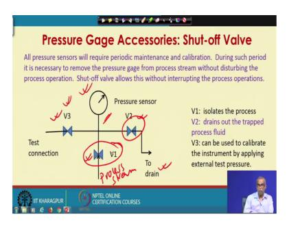
So, let us take a quick look at some pressure gage accessories. Shut-off valve; all pressure sensors will periodic maintenance and calibration. During such period it is necessary to remove the pressure gage from process stream without disturbing the process operations, process operation must go on and we need to isolate the pressure
