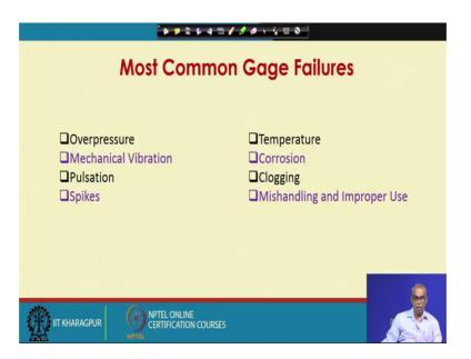
These are common gage failures; overpressure, mechanical, vibration, pulsation, spikes, temperature, corrosion, clogging, mishandling and improper use. So, these are certain most common gage failures.
