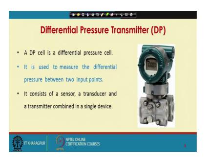
So, let us start our discussion with differential pressure transmitter known as DP cell, what you see is the photograph of a DP cell. So, DP cell is a differential pressure cell, so it measures delta P or difference between two pressures. So, you will see here that there will be connections for two different pressure sources. A DP cell is used to measure the differential pressure between two input points. It consists of a sensor a transducer and a transmitter combined in a single device.
